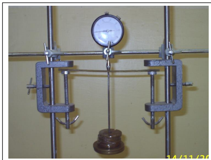
Figure (1): Flexural Apparatus with Specimen Test.
