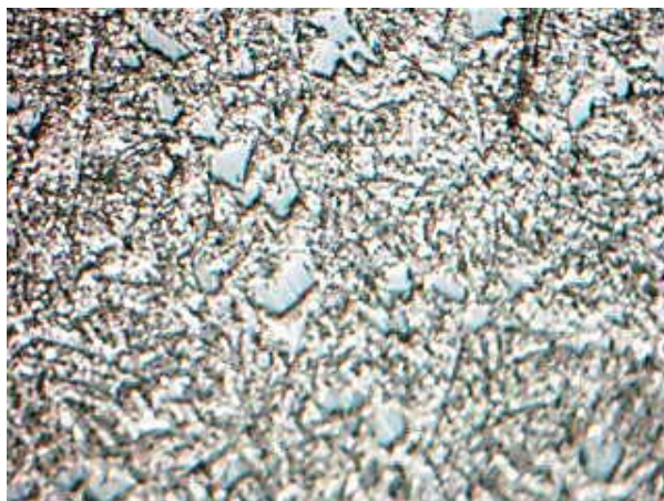
Fig.3 Al-20Si modified by Sr (sample 2) x200
