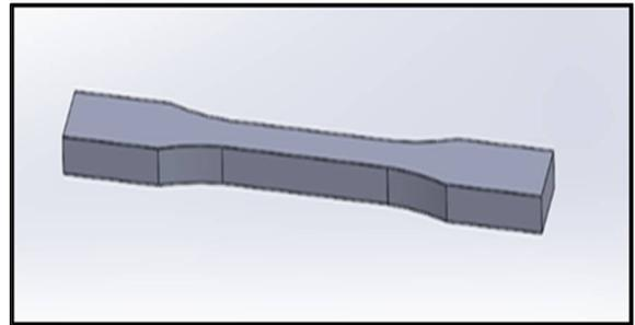
Figure 4: SolidWorks model of the parts specimen
