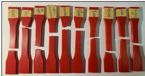
**Figure 9:** Specimens after tensile test
