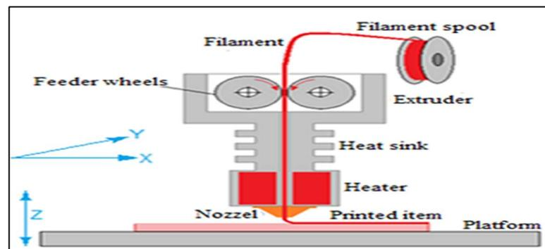
Figure 1: Principle of fused deposition modelling
