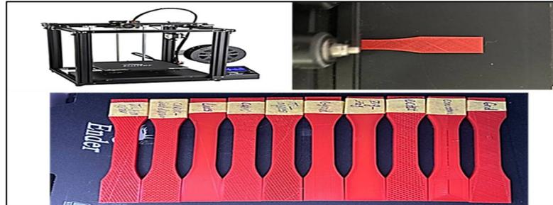
**Figure 8:** 3D printing of infill pattern of test specimen on (Ender 5) 3D printer
