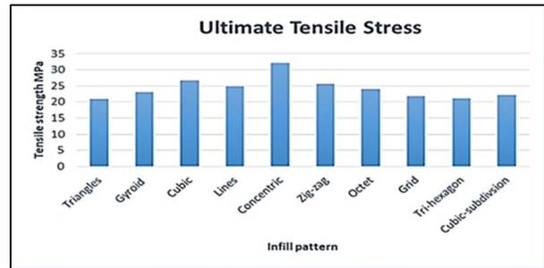
**Figure 10:** Tensile Strength vs. Infill Pattern
