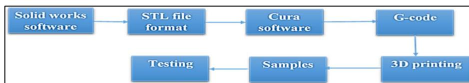
Figure 7: Diagram Flow Chart of Experiment
