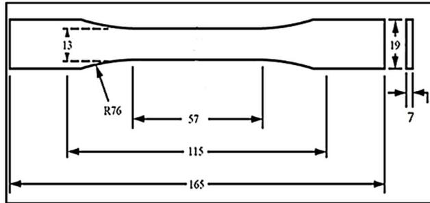
Figure 3: Dimensions used for 3D printed tensile specimen [18]
