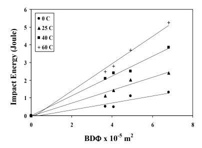
Fig. 3: Impact energy - BDΦ curve for glass fiber reinforced epoxy.
