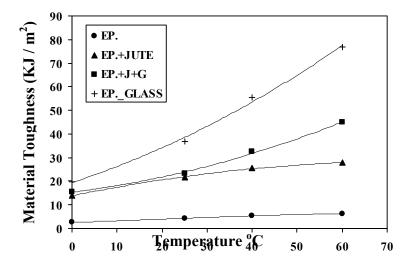
Fig. 5: Material Toughness-Temperature Curve.
