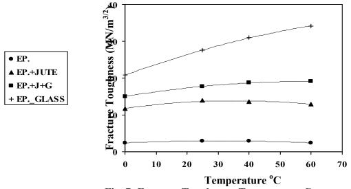
Fig. 7: Fracture Toughness-Temperature Curve.
