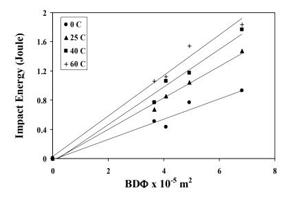
Fig. 2: Impact energy - BDΦ curve for jute fiber reinforced epoxy.
