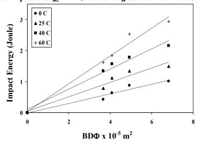
Fig. 4: Impact energy - BDΦ curve for hybrid fiber (15% glass + 15% jute) reinforced epoxy.
