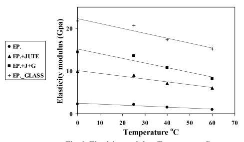
Fig. 6: Elasticity modulus- Temperature Curve.
