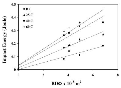
Fig. 1: Impact energy - BDΦ curve for unreinforced epoxy.
