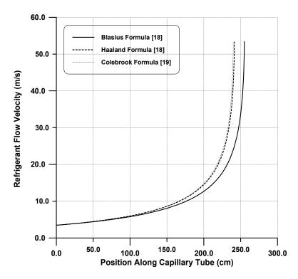
Figure (6): The present model predicted refrigerant (R-22) velocity profile for Sami et al. [21] operating conditions of the capillary tube.
