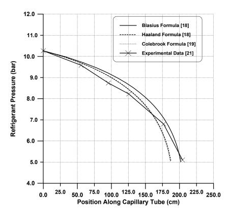
Figure (8): Comparison of predicted pressure profile for refrigerant (R-407C) of the present model with Sami et al. [21].
