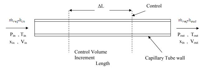
Figure (1): A Schematic diagram for the control volume of fluid flowing inside the capillary tube.
