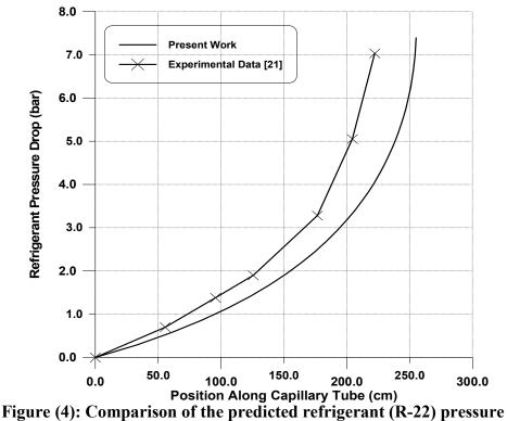
drop profile with the experimental data of Sami et al. [21].
