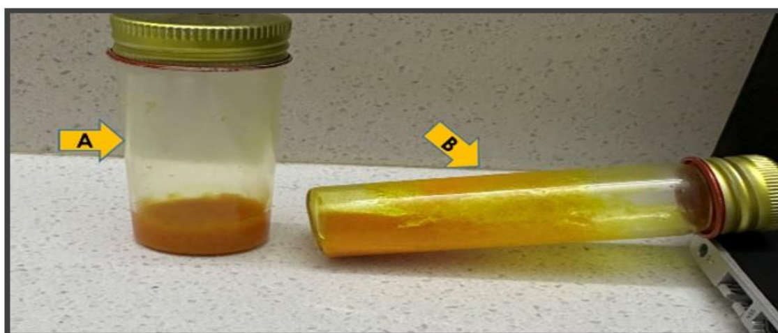
Figure 2: Thermal behavior of the organogels (A) Semi-solid state of the organogel at room temperature and (B) sol state of the organogel at 39 °C and above temperature.
