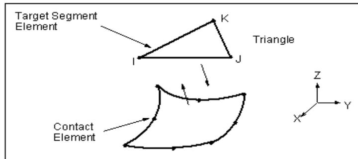
(Fig.3) Targe170 target surface element.
