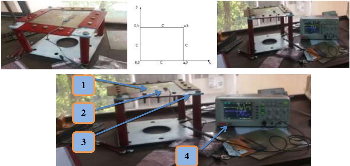
(Fig.1) free vibration techniques with all edges are clamped (CCCC).
