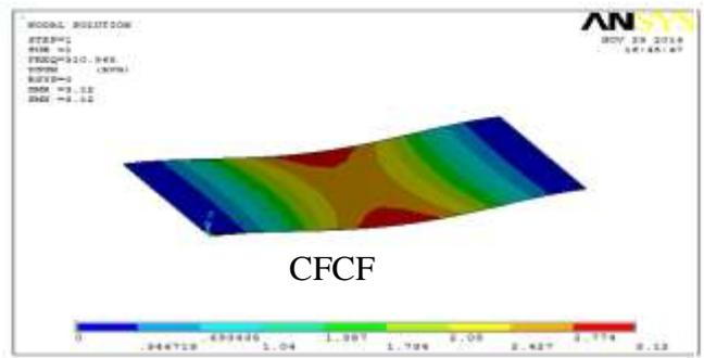
(Fig.8) : fundamental Mode shape for free vibration of symmetric cross ply laminated plates (0/90/90/0) of (CCCC) and (CFCF) plate by Ansys .
