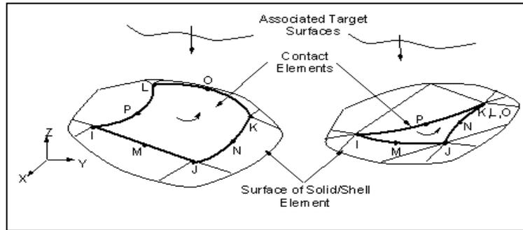
(Fig.4) Conta174 3-D surface-to-surface contact element (8-node).
