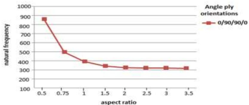
(Fig.12) : Variation of nonlinear fundamental natural frequency with aspect ratio for cross-ply (0/90/90/0) for (CCCC).
