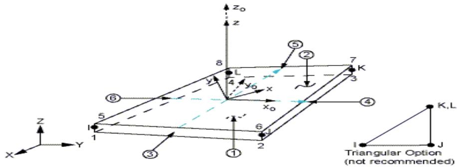
(Fig.2) shell181 Geometry
