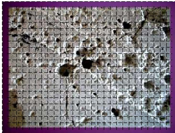
Fig4: Finite element mesh for video image (4-node element)
