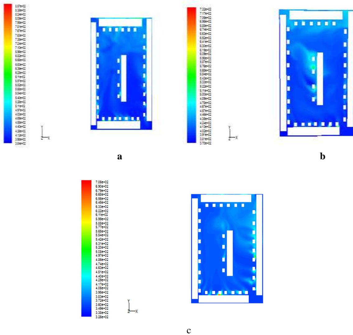
**Fig. 8** Contour of contaminate concentration at seven poles with  $y=0.4\text{m}$  for laboratory:
