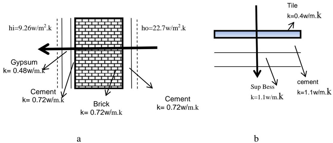
**Fig.2** (a) Heat transfer through the wall, (b) Heat transfer through the floor.
