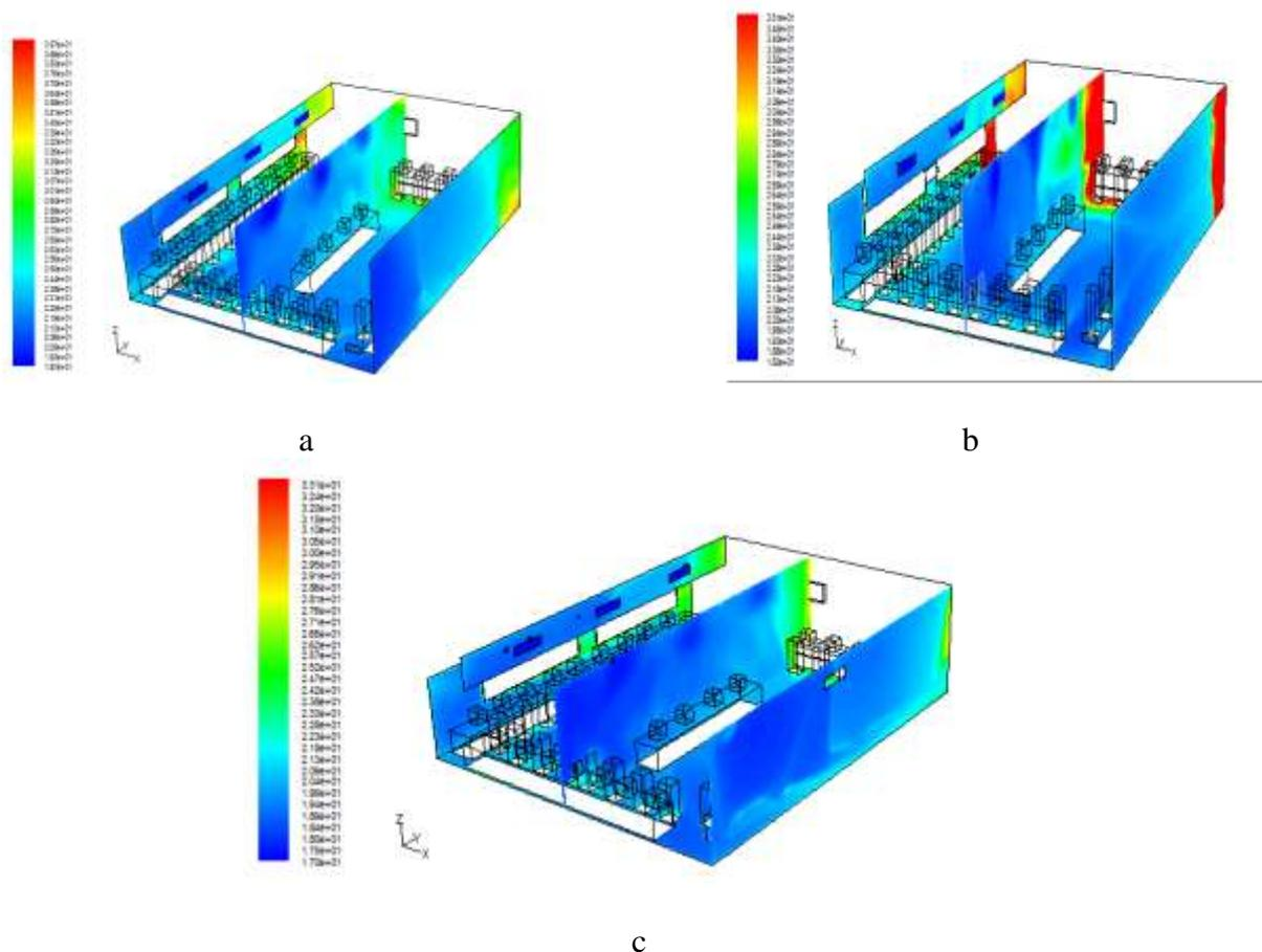
**Fig.5** Distribution of air temperature contours for Plane at  $x=5\text{m}$ , (a) case-I, (b) case-II, (c) case-III
