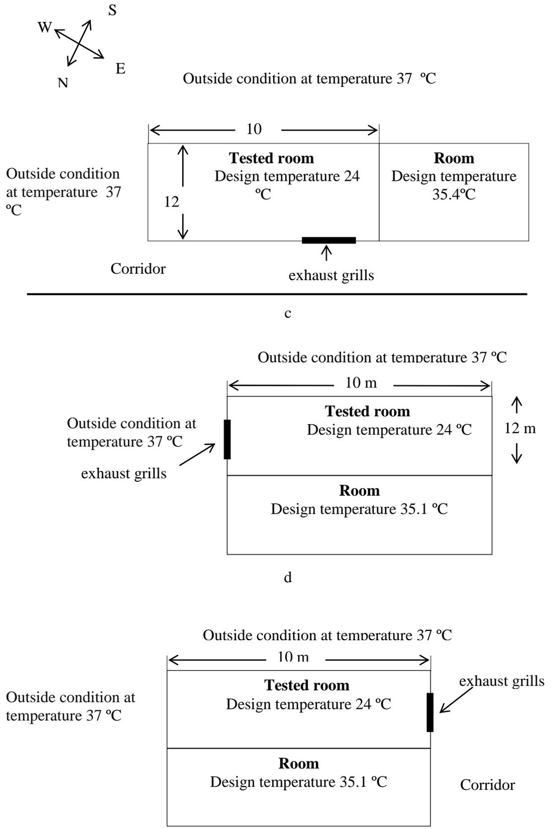
**Fig. 1** (a) Photograph of computer laboratory adopting MV system. (b) Schematic diagram for tested room (Case-I). (c) Schematic diagram for tested room, (Case-I). (d) Schematic diagram for tested room (Case-II). (e) Schematic diagram for tested room, (Case-III).
