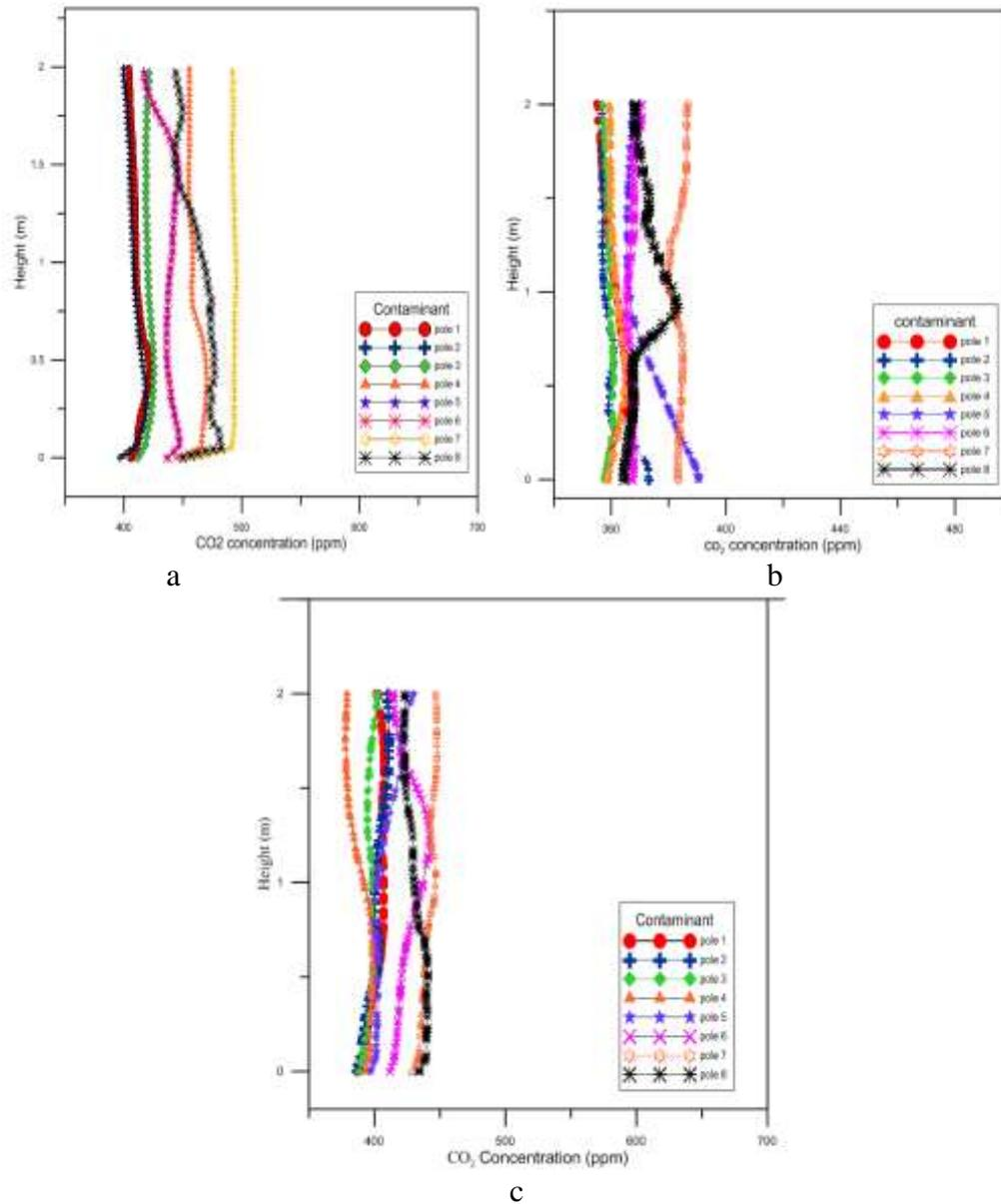
**Fig. 7** CO<sub>2</sub> concentration with height at seven poles for laboratory:
