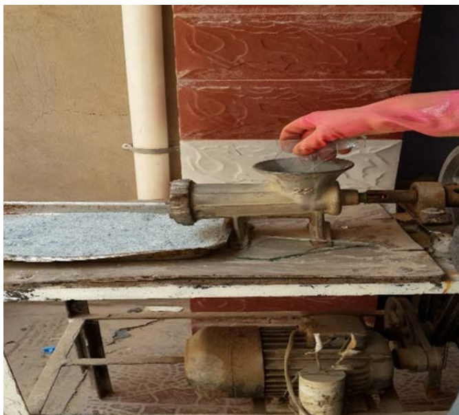
Fig. 1: Glass crushing by electric grinder machine
