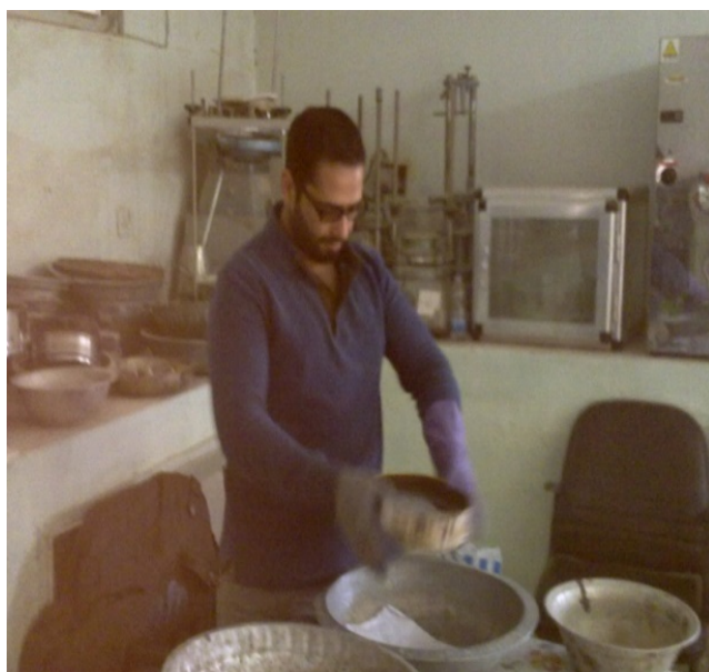
Fig. 2: Sieving process for glass
