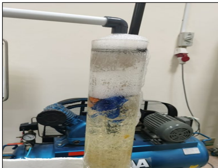
Figure 12: A picture of the rising foams in the counter-current-packed column scheme
