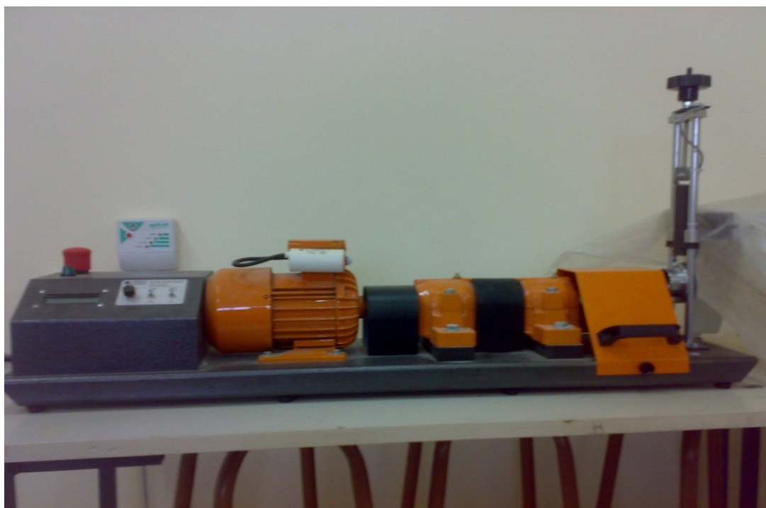
Fig. (1) shows the testing device for fatigue bending rotor technology used in the practical field of search
