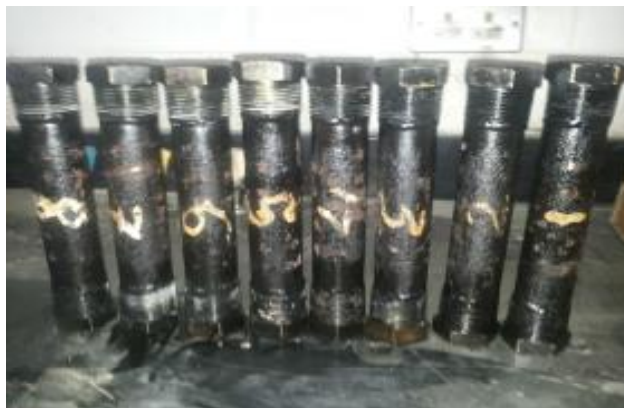
Fig. 3. Core holder of the fluid injection system
