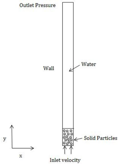
**Fig. 1: The fluidized bed column setup with 1 m height and 0.0254 m diameter.**
