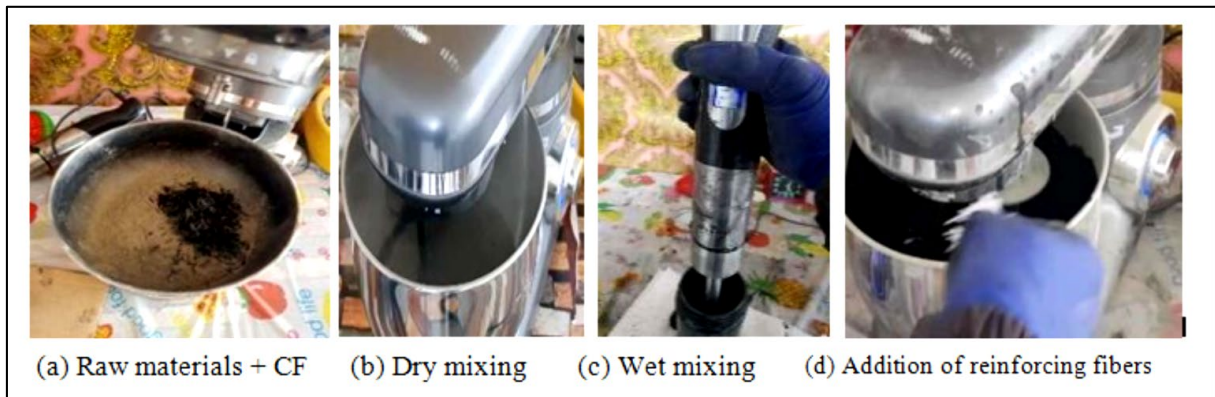
Figure 3: Mixing steps of cementitious composites
