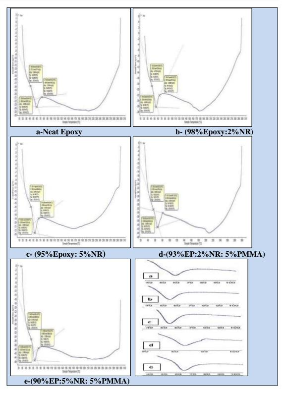
Fig (17) DSC images illustrating of (Tg) values for(a) neat epoxy, binary polymer blend(b) (EP-2%NR),(c) (EP-5%NR), ternary polymer blend(d) (EP: 2%NR: 5%PMMA) and(e) (EP: 5%NR: 5%PMMA)
