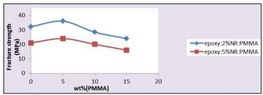
**Fig (5)** Fracture strength for ternary polymer blend (Epoxy: 2 or 5 %NR: X% PMMA) as a function of PMMA content in the blend .
