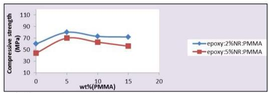
Fig (13) Compressive strength for ternary polymer blend (Epoxy: 2 or 5 %NR: X% PMMA) as a function of PMMA content in the blen
