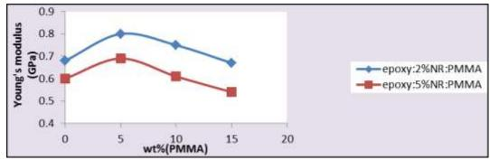
**Fig (6)** Young's modulus for ternary polymer blend (Epoxy: 2 or 5 %NR: X% PMMA) as a function of PMMA content in the blend .
