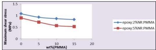
Fig (10) Maximum shear stress for ternary polymer blend (Epoxy: 2 or 5 %NR: X% PMMA) as a function of PMMA content in the blend.
