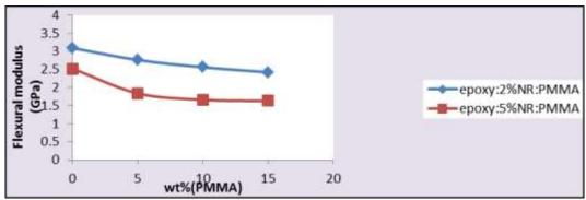
Fig (9) Flexural modulus for ternary polymer blend (Epoxy: 2 or 5 %NR: X% PMMA) as a function of PMMA content in the blend .
