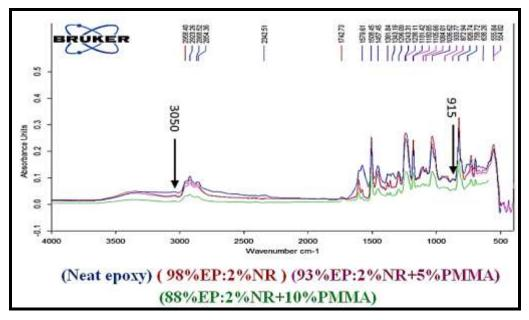
**Fig** (1) FTIR spectrum of ternary polymer blend (Epoxy-NR - PMMA) as a function of PMMA content in the blend
