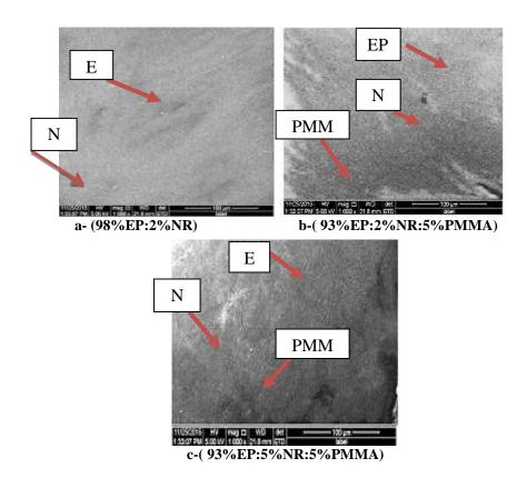
**Fig (18 a, b, c and d)** SEM Images Showing the effect of addition (5%PMMA) on the Surface Morphology of polymer blend (98%EP: 2%NR) at Magnification (X=1000)
