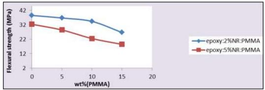
**Fig (8)** flexural strength for ternary polymer blend (Epoxy: 2 or 5%NR: X% PMMA) as a function of PMMA content in the blend.
