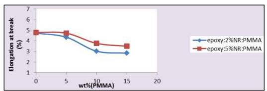
Fig (7) Elongation at break for ternary polymer blend (Epoxy: 2 or 5 %NR: X% PMMA) content in as a function of PMMA the blend
