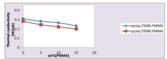
Fig (15) Thermal conductivity for ternary polymer blends (Epoxy: 2 or 5 %NR: X% PMMA) as a function of PMMA content in the blend.
