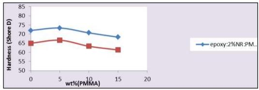
Fig (14) Hardness for ternary polymer blend (Epoxy: 2 or 5%NR: X% PMMA) as a function of PMMA content in the blend
