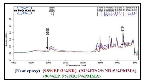
Fig (2) FTIR spectrum of binary polymer blend (98%EP: 2%NR) and ternary blend (Epoxy: X%NR: 5%PMMA), as a function of NR content in the blend (93%EP: 2%NR: 5%PMMA) and (90%EP: 5%NR: 5%PMMA)
