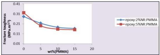
**Fig (12)** fracture toughness for ternary Polymer blend (Epoxy: 2 or 5 %NR: X% PMMA) as a function of PMMA content in the blend
