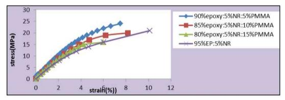
Fig (4) Stress-strain curves for ternary polymer blends (epoxy: 5%NR: X% PMMA) as a function of PMMA content in the blend
