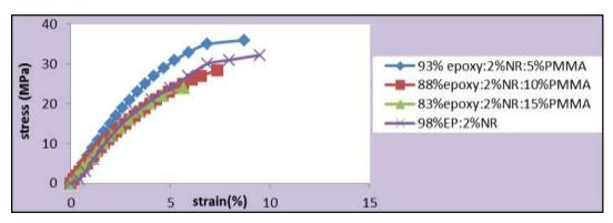
Fig (3) Stress-strain curves for ternary polymer blends (epoxy: 2%NR: X% PMMA) as a function of PMMA content in the blend
