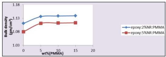
Fig (16) Bulk density for ternary polymer blend (Epoxy: 2 or 5 %NR: X% PMMA) as a function of PMMA content in the blend.
