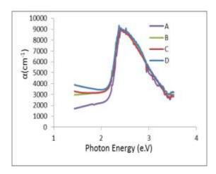
**Fig.(3**): Absorption coefficient spectra for PVC doped with DCM thin films mixed with different particle density of TiO<sub>2</sub>.
