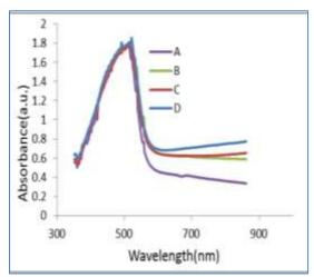
**Fig.(1)**: Absorbance spectra for PVC doped with DCM thin films mixed with different particle density of TiO<sub>2</sub>.
