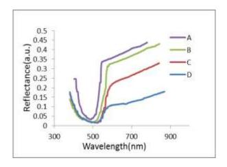
**Fig.(2)**: Reflectance spectra for PVC doped with DCM thin films mixed with different particle density of TiO<sub>2</sub>.
