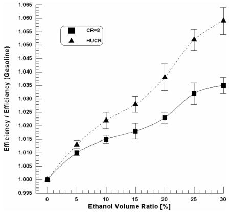
Fig.7. Effect of ethanol blending on the brake thermal efficiency of the Ricardo E6 SI engine.
