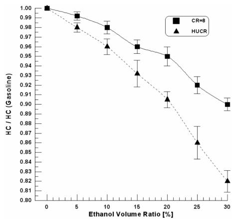
Fig.11. Effect of ethanol blending on the HC of the Ricardo E6 SI engine.
