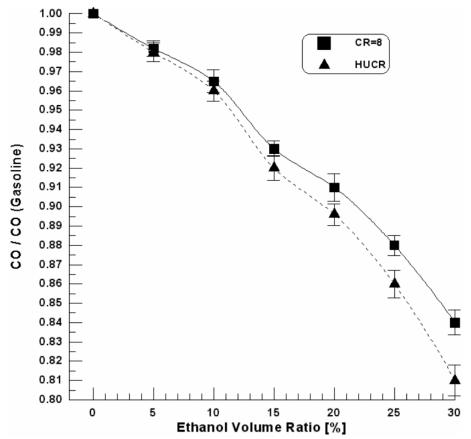
Fig.10. Effect of ethanol blending on the CO of the Ricardo E6 SI engine.
