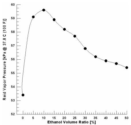
Fig.4. Effect of ethanol blending on the Reid vapor pressure value.
