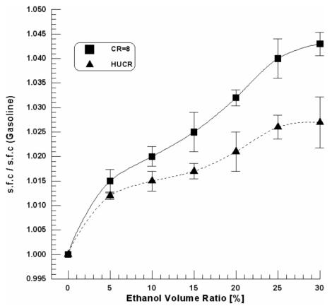
Fig.8. Effect of ethanol blending on the brake specific fuel consumption of the Ricardo E6 SI engine.
