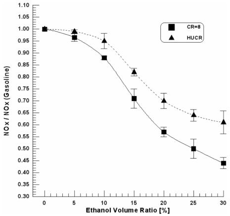
Fig.9. Effect of ethanol blending on the NOx of the Ricardo E6 SI engine.
