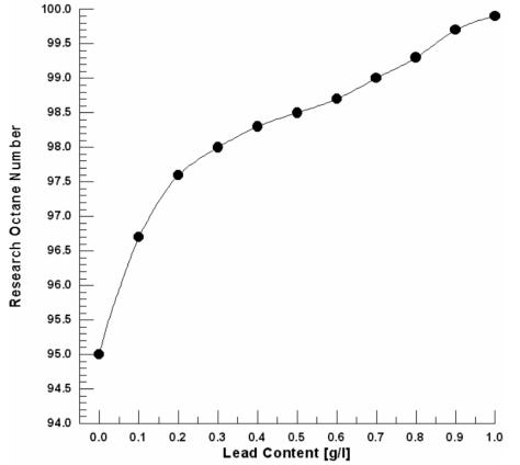
Fig.1. Contribution of lead additives to gasoline octane (RON) for gasoline's (CFR engine).
