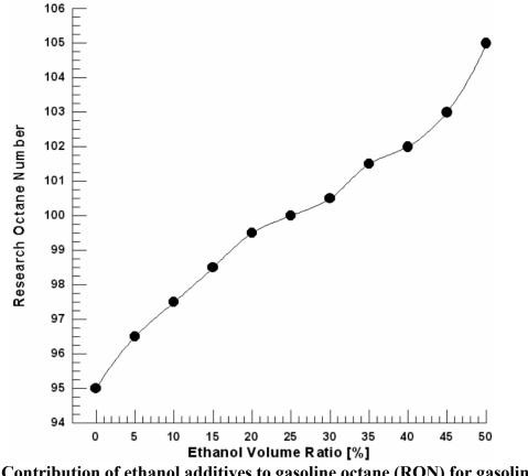
Fig.3. Contribution of ethanol additives to gasoline octane (RON) for gasoline's (CFR engine).
