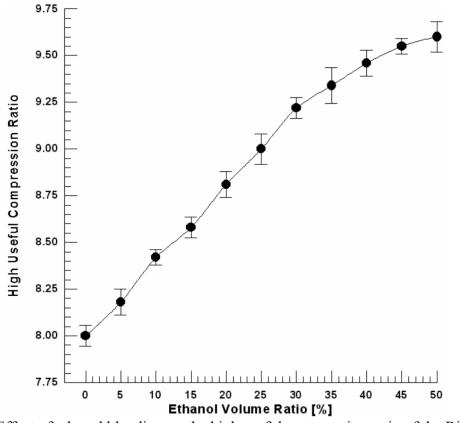
Fig.5. Effect of ethanol blending on the high useful compression ratio of the Ricardo E6 SI engine.
