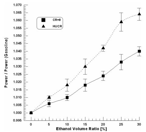
Fig.6. Effect of ethanol blending on the brake power of the Ricardo E6 SI engine.
