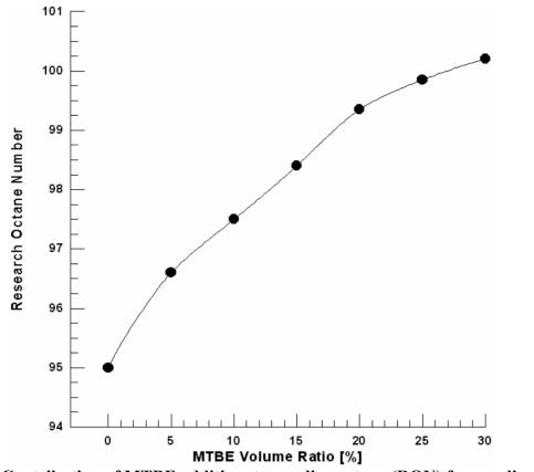
Fig.2. Contribution of MTBE additives to gasoline octane (RON) for gasoline's (CFR engine).
