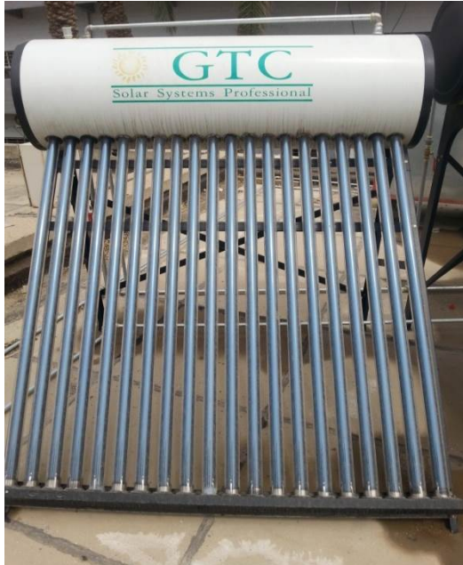
Fig 3. The experimental evacuated tube solar collector
