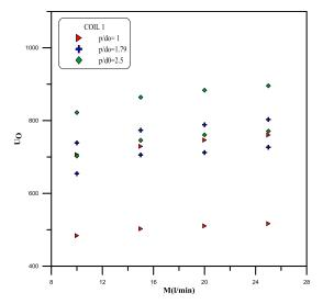
**Fig. (3):** Effect of the coil pitch on the overall heat transfer coefficient for coil 1
