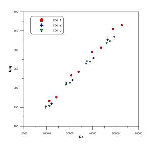
**Fig. (5) : I**nner Nusselt number versus Reynolds number for different Curvature ratio
