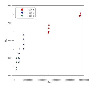
**Fig. (6) :** Outer heat transfer coefficient versus Rayleigh number for different curvature ratio
