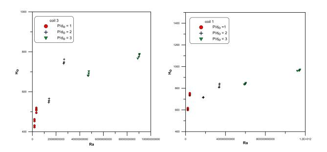
**Fig. (9) :** Effected of the coil pitch on the outer heat transfer coefficient for coil 3
