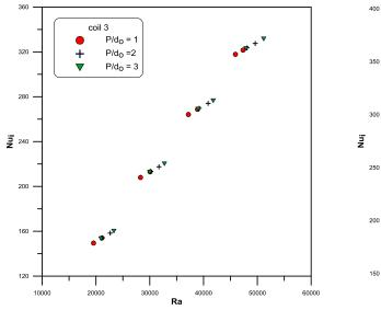
**Fig.** (7) : effect of the coil pitch on inner Nusselt number for coil 3
