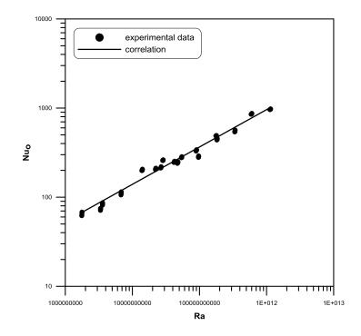
Fig. (11) : Average turbulent heat transfer correlation for vertical coils in water with coil height as a characteristic length
