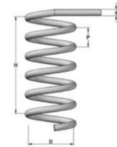
Fig. (2): physical Dimensions of this Coil
