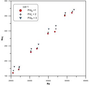
**Fig. (8) :** effect of the coil pitch on the inner Nusselt number for coil 1
