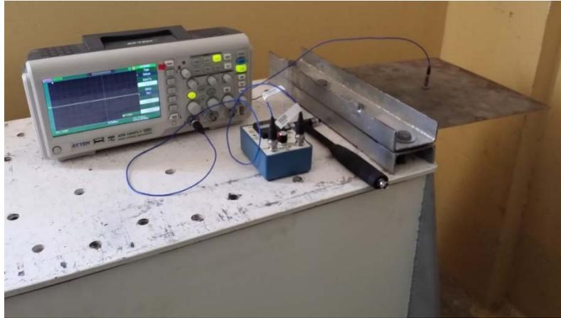
Fig. (3): rig and vibration test of the plate structure
