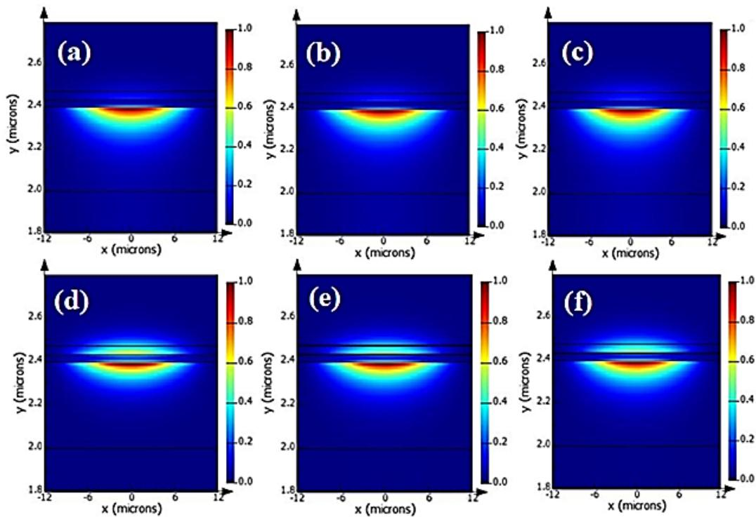
**Figure 5:** The increasing electric field: (a) Silver without Graphene in  $N=1.1$ . (b) Silver without Graphene in  $N=1.2$ . (c) Silver without Graphene in  $N=1.3$ . (d) Silver with graphene thickness of 1 nm and  $N=1.1$ . (e) Silver with graphene thickness of 3 nm. (f) Silver with graphene thickness of 5 nm
