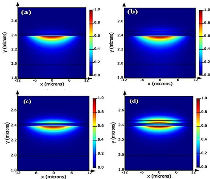
Figure 4: Silver layer: (a) Silver without Graphene in air. (b) Silver without Graphene in water. (c) Silver with Graphene in air. (d) Silver with Graphene in water
