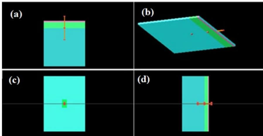
**Figure 1:** The proposed SPR sensor design: (a) afront view. (b) top view (c) left view. (d) right view
