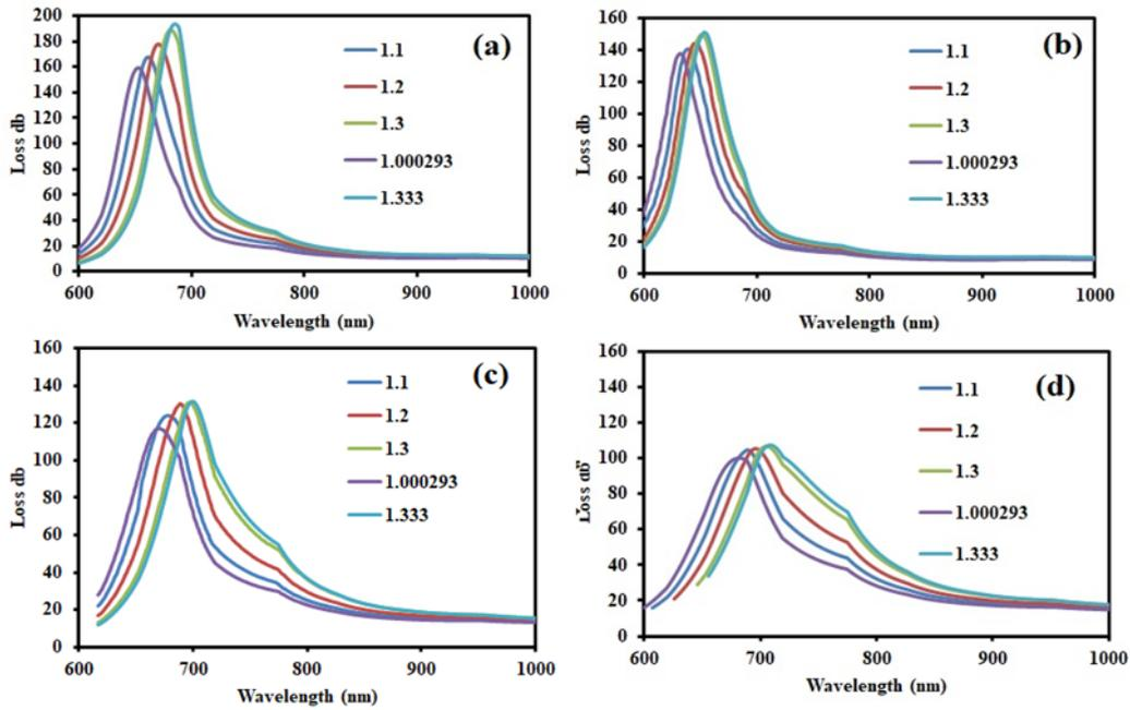
Figure 2: Analyte refractive index with thickness silver metal (30 nm) (a without graphene b) graphene 1 nm thickness (c graphene 3 nm thickness d) with graphene 5 nm thickness
