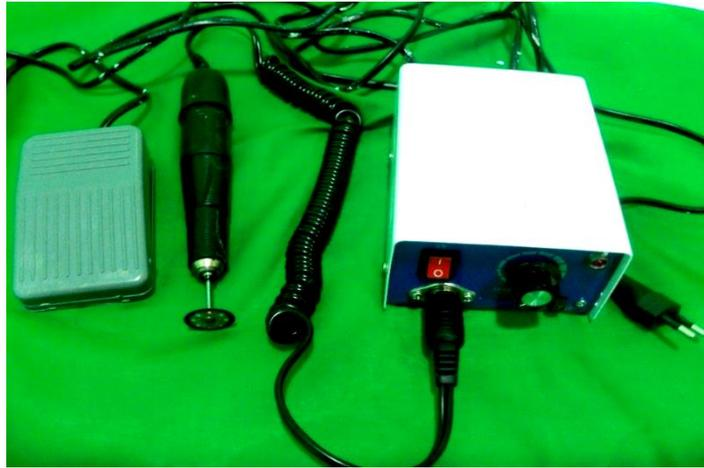
**Figure 2:** Electrical rotating saw with 10 mm width and 0.5 mm thickness blade used for osteotomy.
