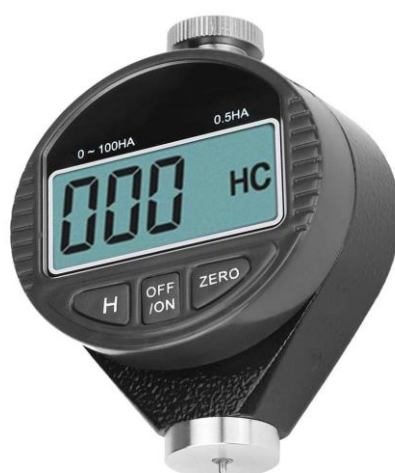
Figure 2: Durometer instrument used in the study
