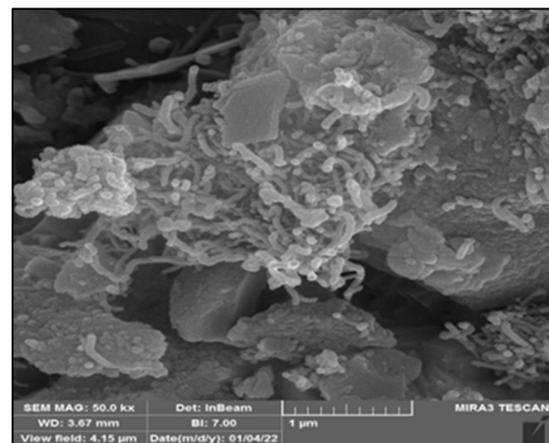
Figure 6: SEM image of the G2 sample containing CNTs
