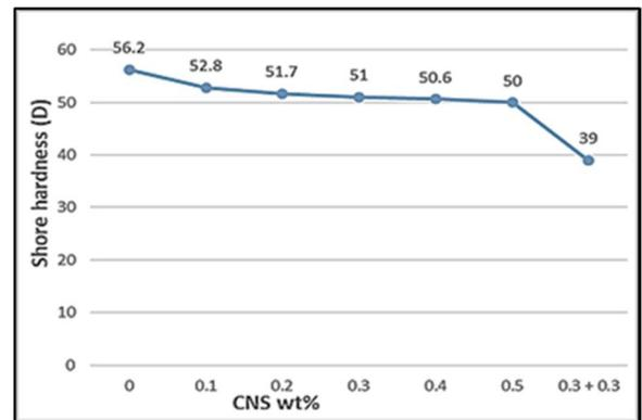
Figure 14: Effect of the addition of CNSs on the hardness of the G3 sample
