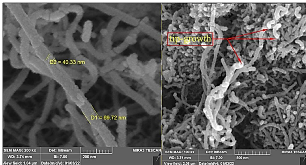
Figure 4: (98% Pure CNTs prepared by the arc discharge method
