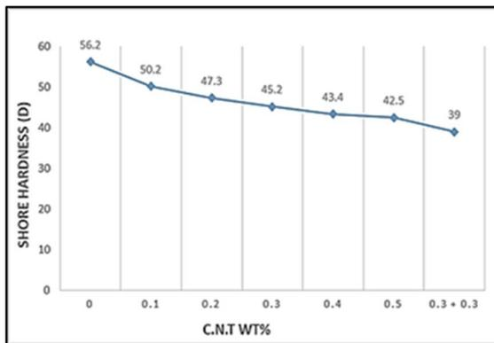
Figure 13: Effect of the addition of CNTs on the hardness of the G2 sample
