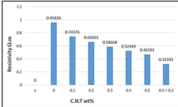
Figure 15: Resistivity of the sample G2 as a function of the CNT wt. % additive
