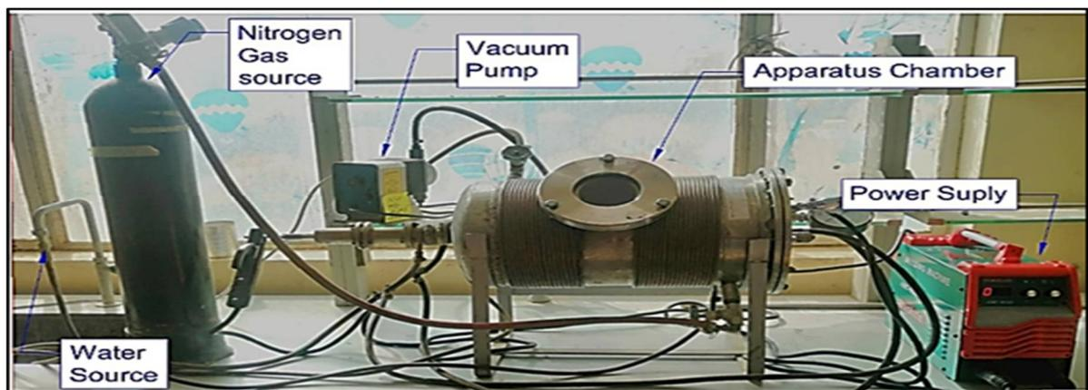
**Figure 2:** The system parts of the arc discharge method
