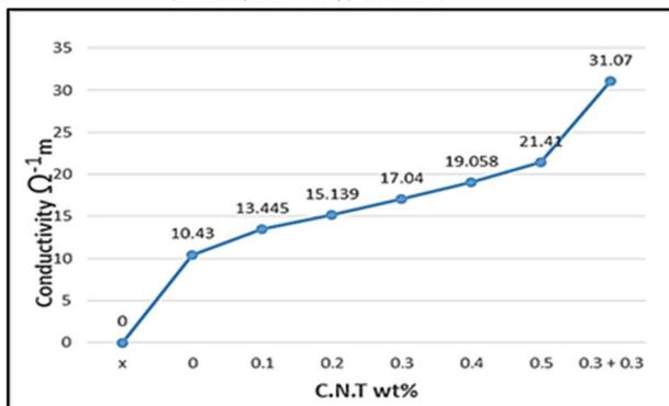
Figure 17: Conductivity of G2 composite as a function of CNT wt. % additive
