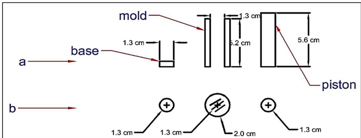
**Figure 3:** (a) Side view of the samples in the mold section, and (b) Front view of the samples in the mold section
