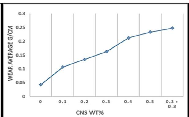
Figure 20: Average wear of the G3 sample as a function of the CNS wt. % additive
