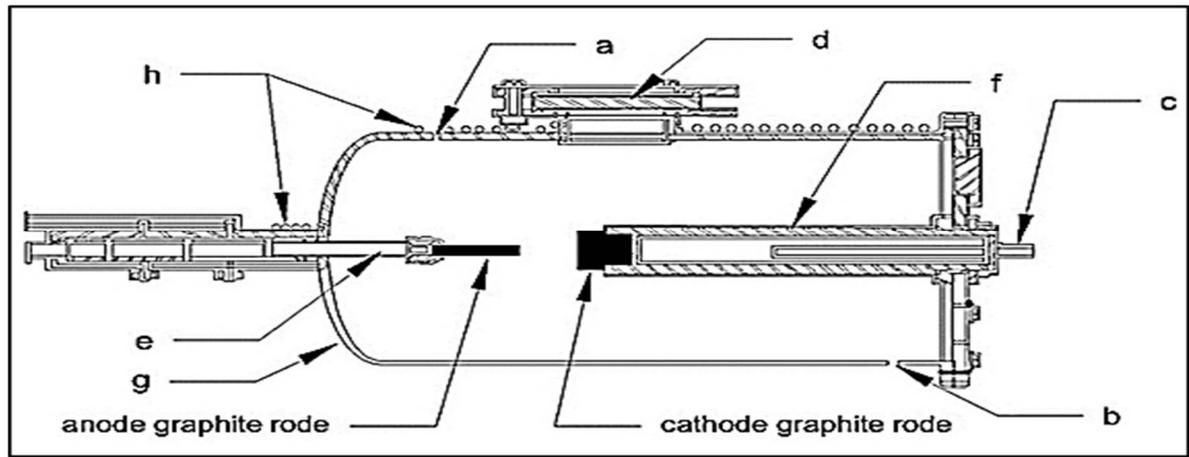
**Figure 1:** Graphical diagram for the arc discharge device: (a) the vacuum way out, (b) gas entry, (c) the inlet and outlet for cathode coolant water, (d) quartz sealed vision window, (e) pure copper shaft coated by nickel, (f) pure copper tube separated from the chamber, (g) chamber of stainless steel, (h) copper cooling water pipes
