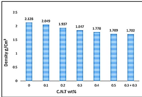
Figure 11: Density of the G2 sample as a function of the CNTs%
