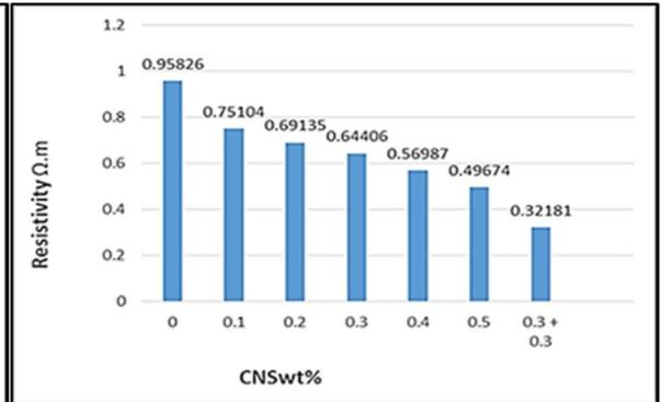
Figure 16: Resistivity of the sample G3 as a function of the CNS wt. % additive
