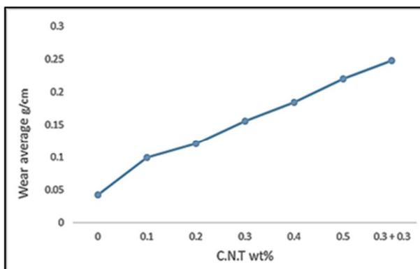
Figure 19: Average wear of the G2 sample as a function of the CNT wt. % additive
