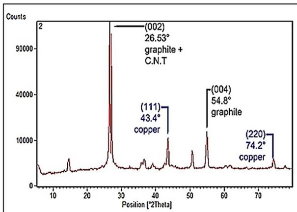
Figure 9: XRD pattern of G2 sample
