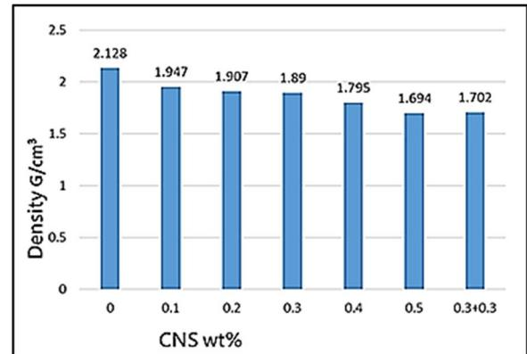
Figure 12: Density of the G3 sample as a function of the CNS%
