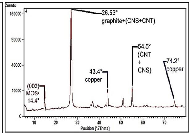
Figure 10: XRD pattern of G4 sample
