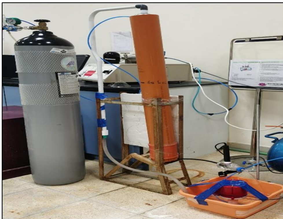
Figure 2: Picture for the gas lift PVC column packed with glass balls and connected to the DO sampling head from the bottom
