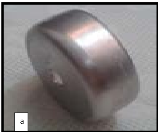
Fig. (29) Formed Cup: (a) Experimentally and (b) Numerically.
