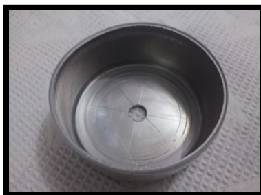
Fig.( 28) Shown the Cup before and after Measuring the Thickness(Thickness 3mm)
