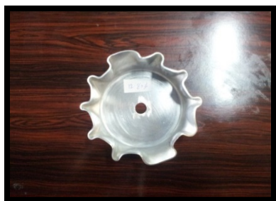
Fig.(27). Shown the Wrinkling(Thickness 2mm)
