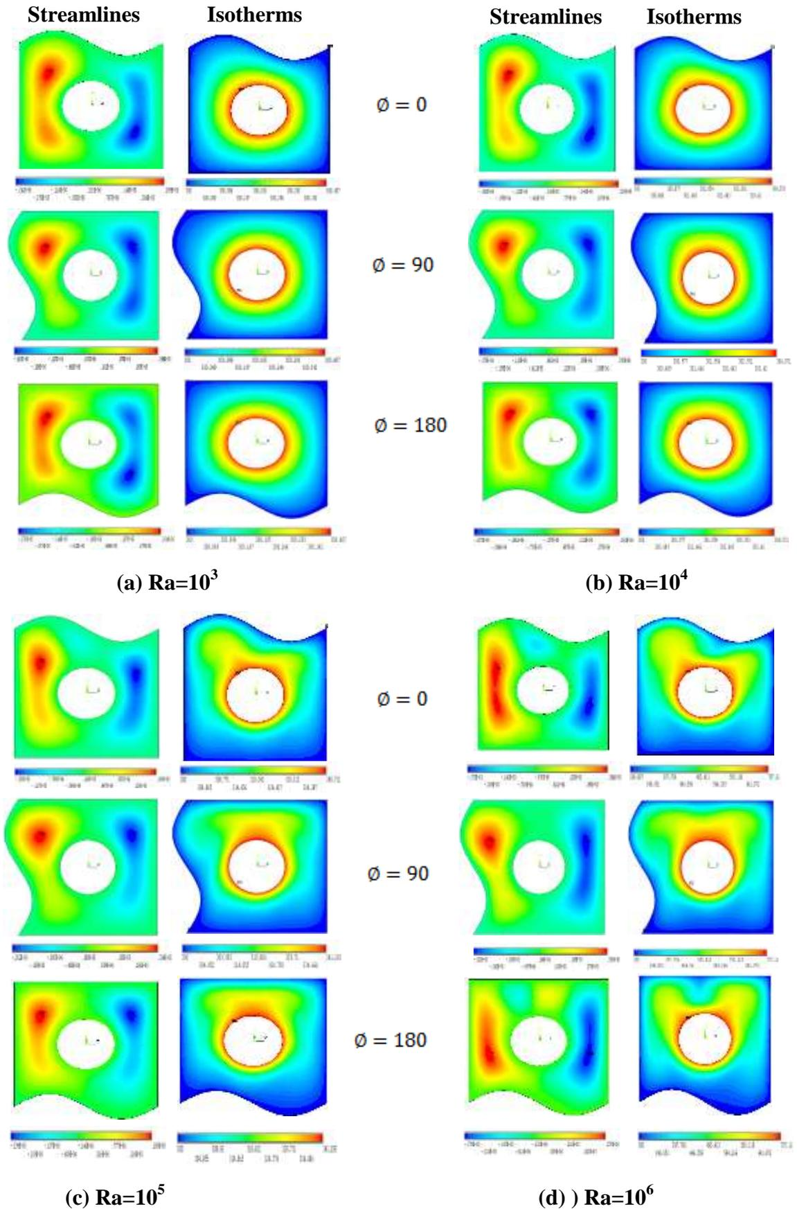
Fig. 4: Variation of streamlines and isotherms with inclination angle for one undulation
