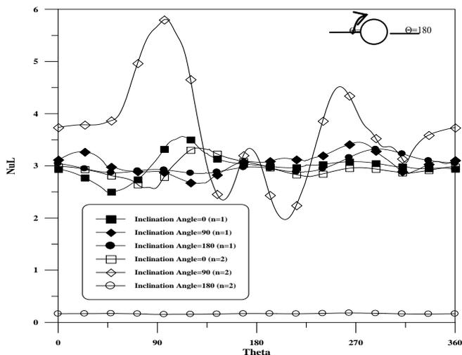
Fig.(6a) Variation of local Nusselt number along heated circular cylinder
