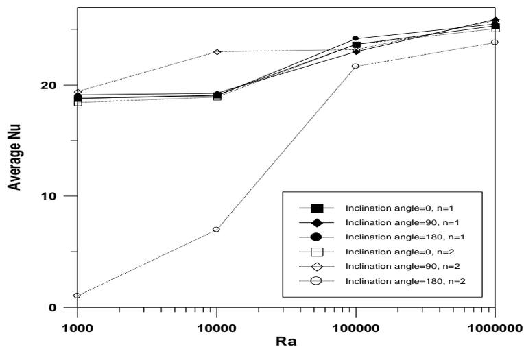
Fig. 7. Average Nu versus Ra with different parameters.
