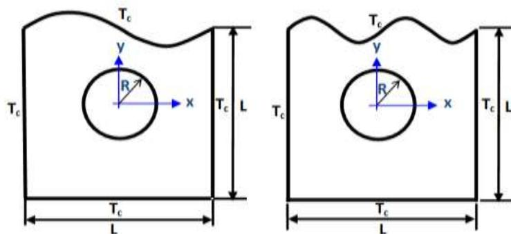
**Fig. 1.** Schematic diagrams of wavy wall enclosure at an inclination angle  $\phi=0^\circ$  for one undulation ( $n=1$ ) and two undulations ( $n=2$ )
