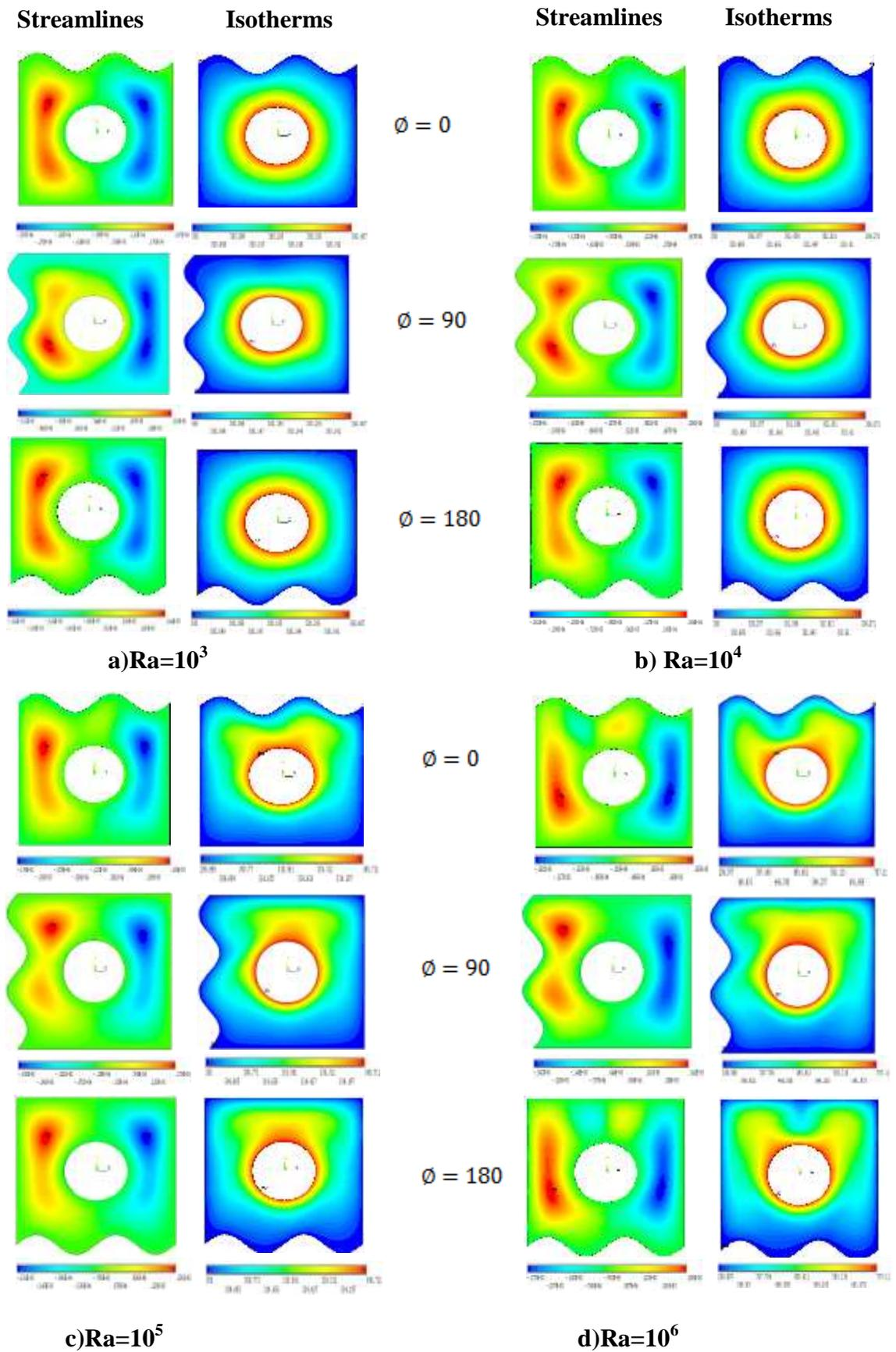
Fig. 5: Variation of streamlines and isotherms with inclination angle for two undulation
