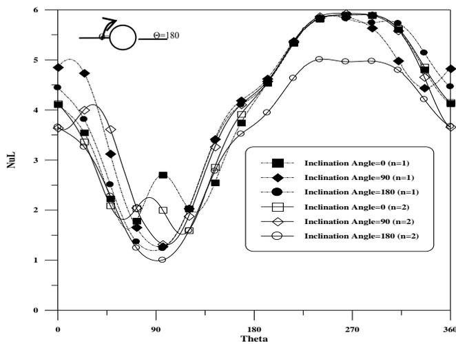
Fig.(6c) Variation of local Nusselt number along heated circular cylinder
