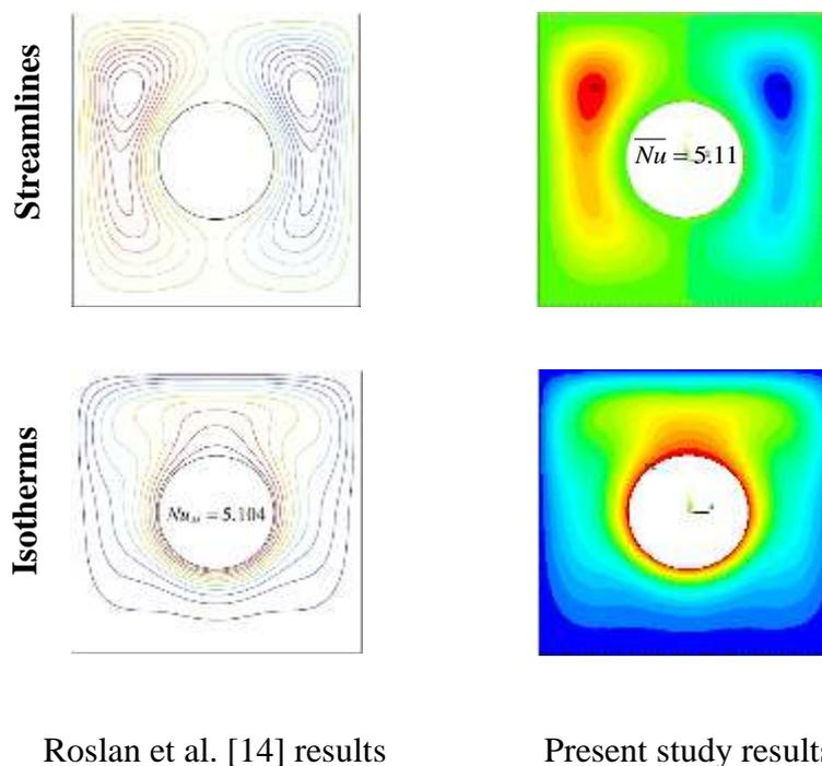
**Fig. 3.** Comparison of the streamlines and isotherms patterns between the percent study (right) and Roslan et al. [14] (left) at  $Ra=10^5$  and  $R=0.2L$ .
