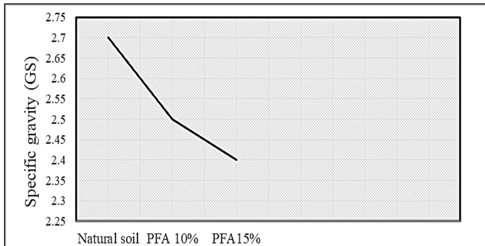
Figure 5: Values of specific gravity for treated and untreated soil
