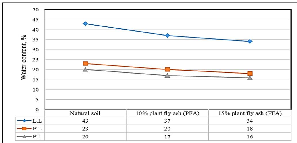
Figure 4: Effect of cement paste and plant fly ash (PFA) content on Atterberg limits
