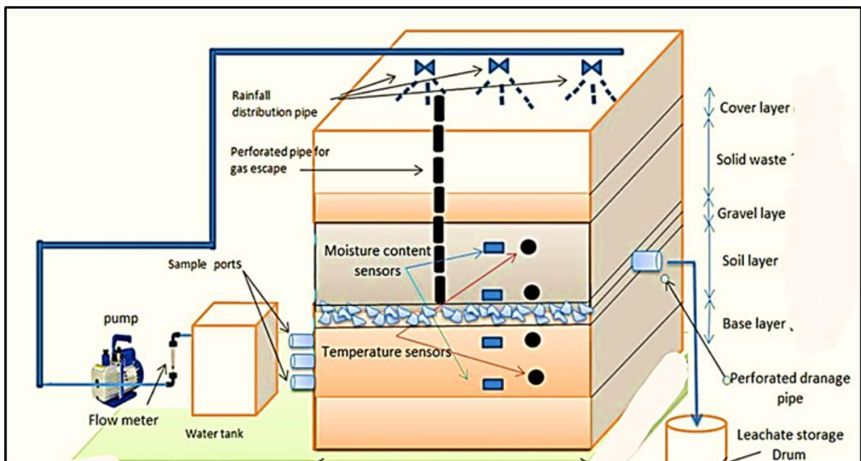
Figure 2: Pilot-scale lysimeter drawing
