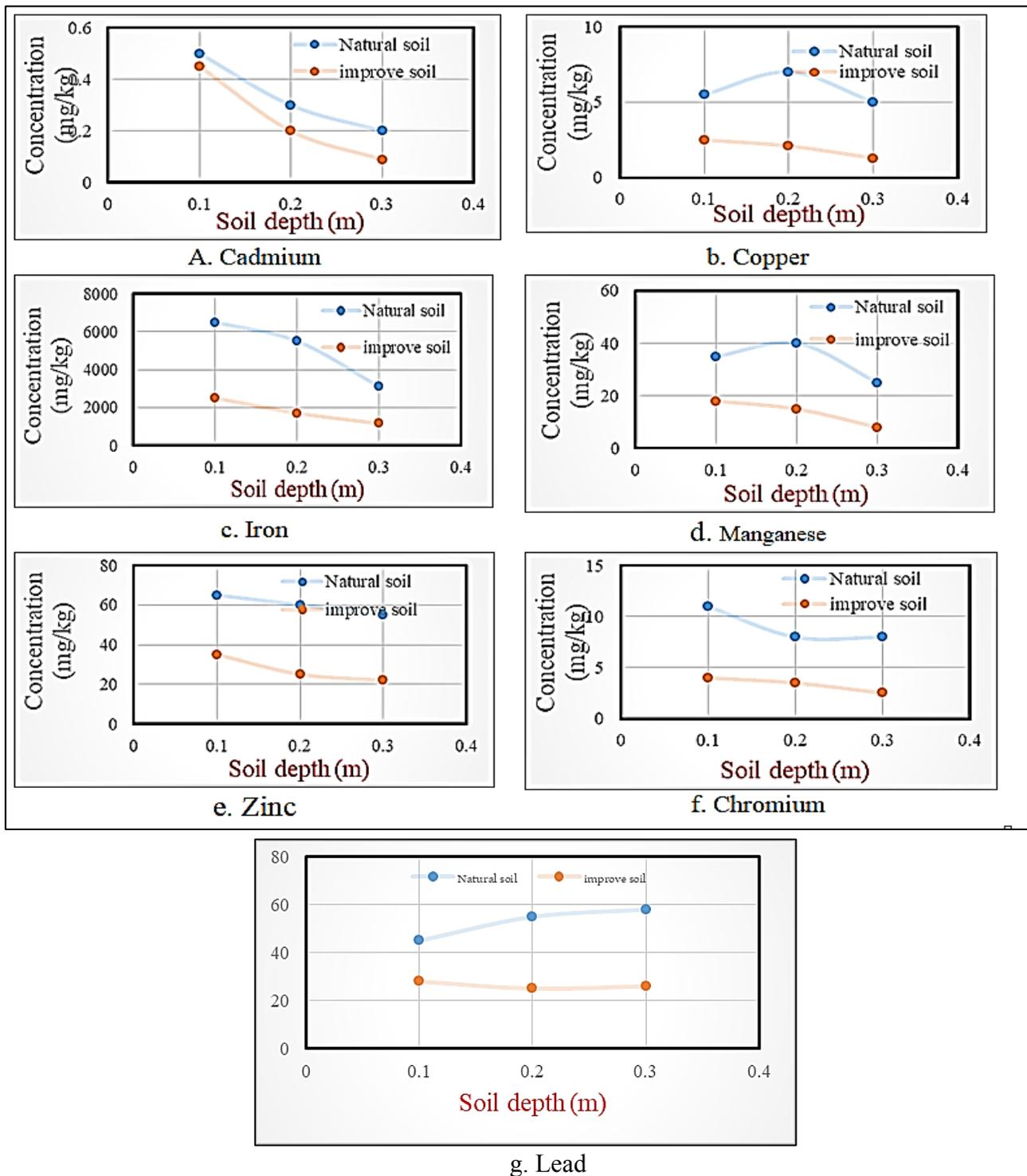
Figure 18: Heavy metal vs. mid-depth of soil samples
