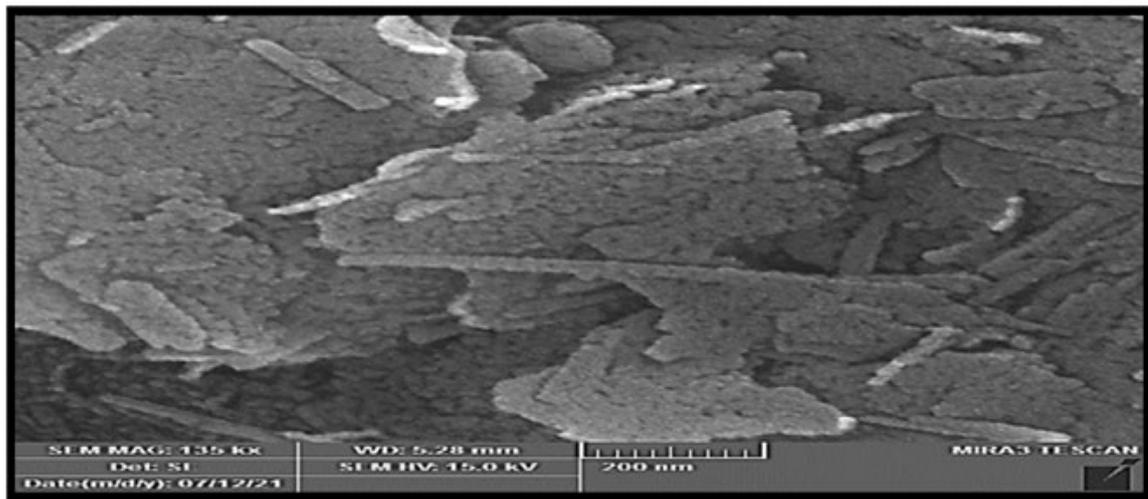
**Figure 11:** The morphology of the sample grains (10% plant fly ash to soil) in a survey range of 200 nm
