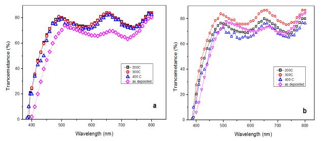
Fig. (5): Optical transmittance of the ITO films annealed at different annealing temperature and atmospheres: (a) in vacuum atmosphere and (b) in oxygen atmosphere
