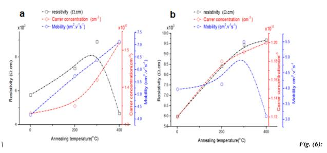
Resistivity of the ITO films annealed at different temperature and atmospheres: (a) in a vacuum atmosphere and (b) in oxygen atmosphere.
