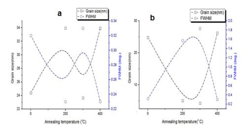
Fig. (3): crystallite size and FWHM of the ITO films annealed in (a) in a vacuum atmosphere and (b) in oxygen atmosphere.
