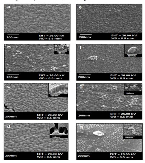
Fig.(4): Scanning electron micrographs of the  $In_2Sn_2O_7$  films, (a) As-deposited, (b, c and d) annealed In a vacuum atmosphere at (200, 300 and 400) °C and (e, f, g and h) annealed in oxygen atmosphere at (200, 300 and 400)°C.
