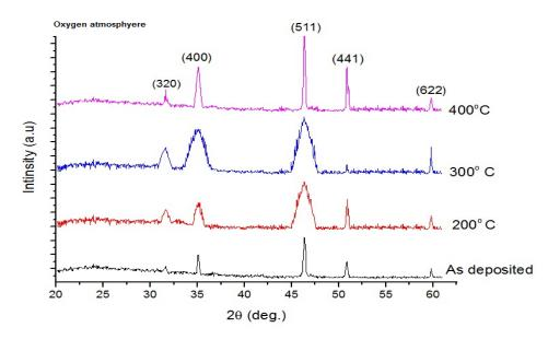
Fig. (2): (XRD) patterns of the ITO films as-deposited and annealed at Oxygen Atmospheres.
