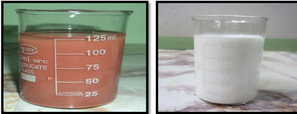
Fig.1 Depicted nanofluids for  $\text{CuO} + (\text{EG} + \text{Dw})$  ,  $\text{TiO}_2 + (\text{EG} + \text{Dw})$
