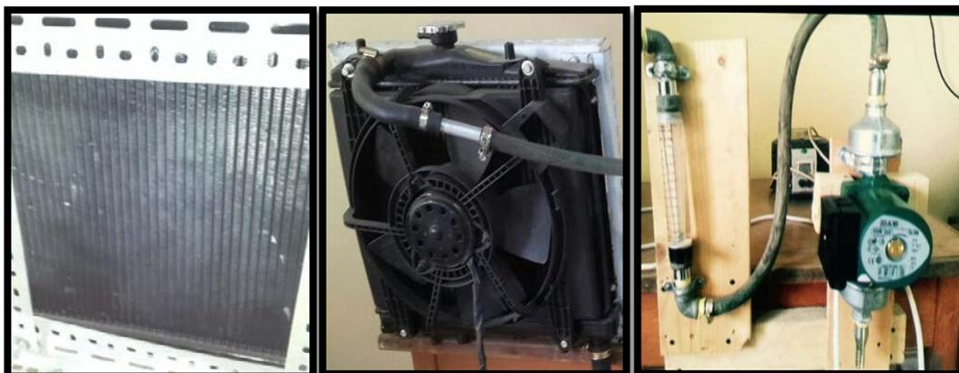
Fig 3. The radiator, flow meter and pump used in the experiments.
