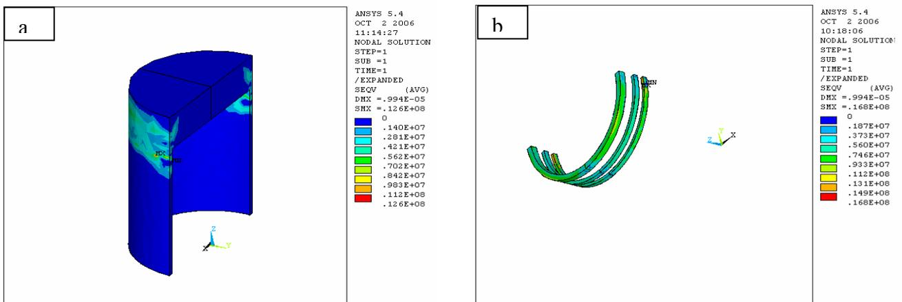
Fig (7) stress distribution a, piston (alloy2) b-rings
