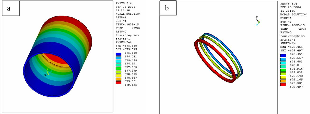
Fig (5) temperature distribution a, piston (alloy3) b-rings
