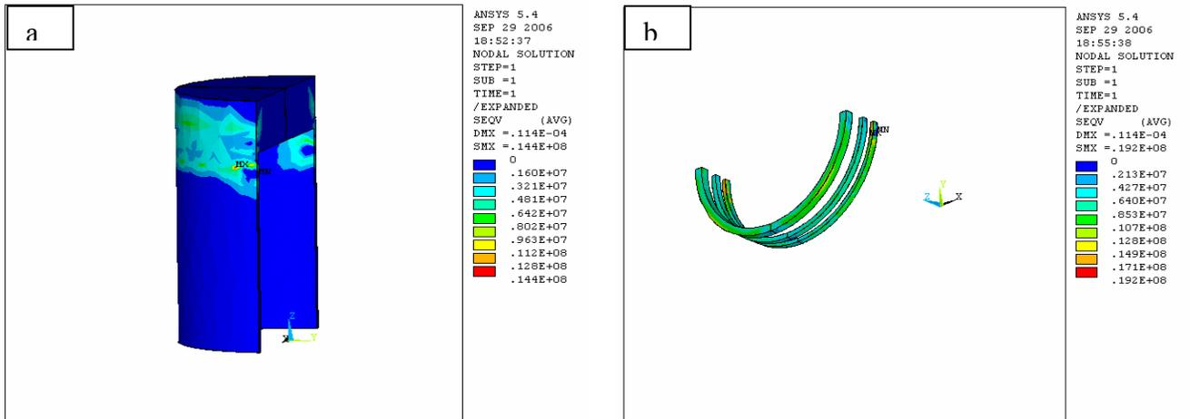
Fig (6) stress distribution a, piston (alloy1) b-rings
