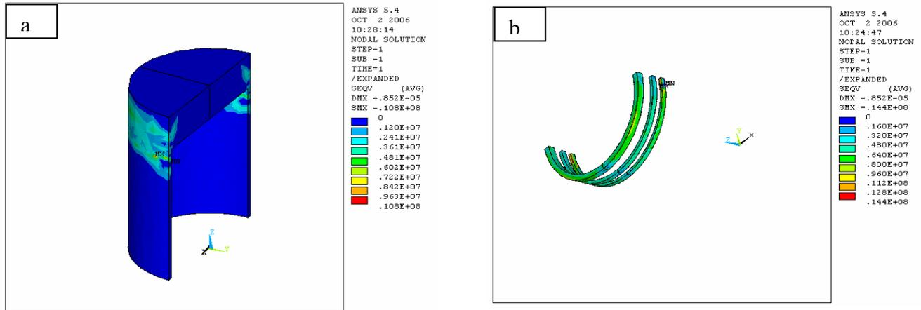
Fig(8) stress distribution a, piston (alloy3) b-rings
