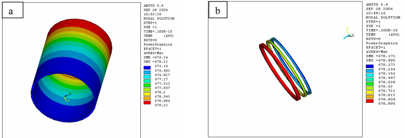
Fig (3) temperature distribution a, piston (alloy1) b-rings
