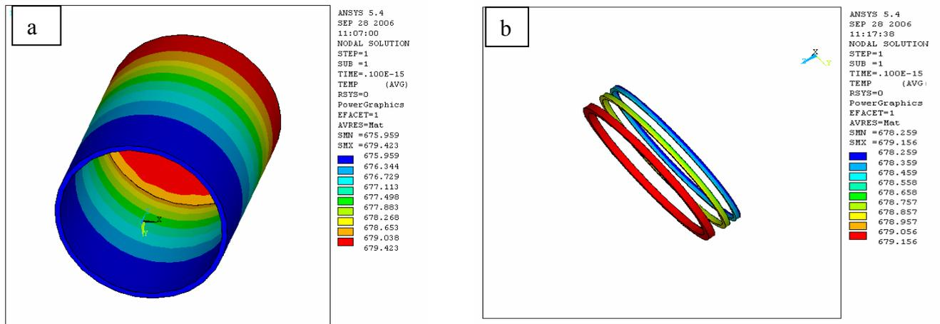
Fig (4) temperature distribution a, piston (alloy2) b-rings
