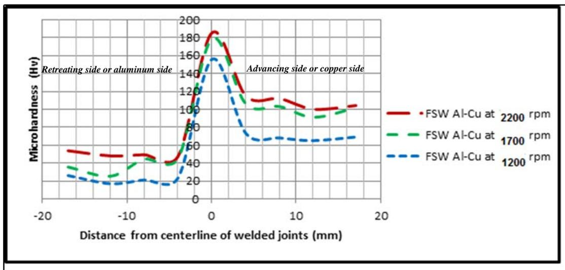
**Figure 7:** The average microhardness profile across the welded joints at three different rotational speeds.
