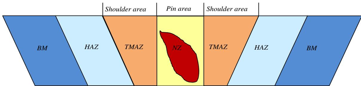
Figure 2: Welding zones after FSW process.
