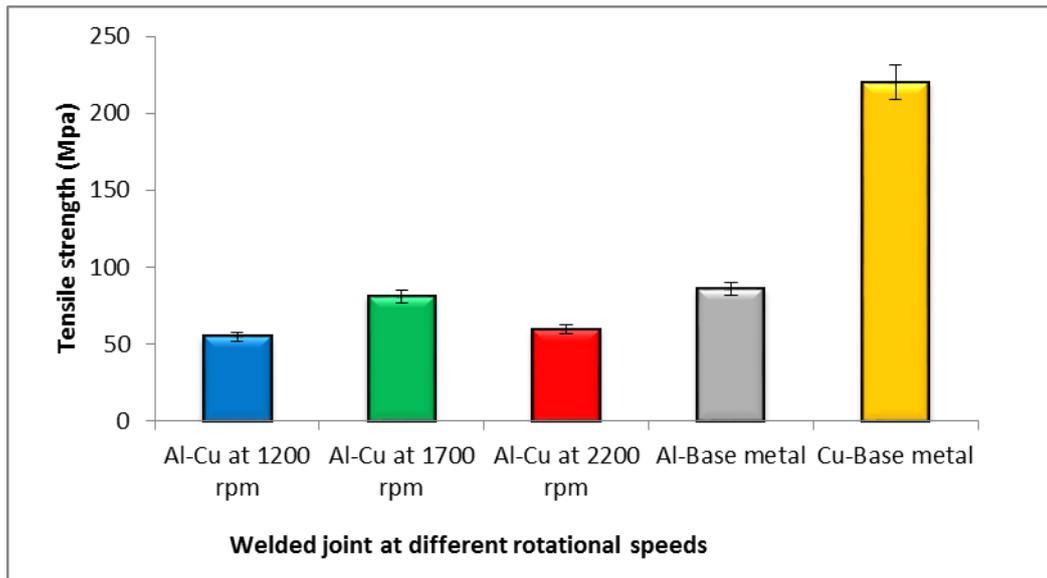
**Figure 8:** Tensile test profiles of the dissimilar Al-Cu welded joints at three different rotational speeds.
