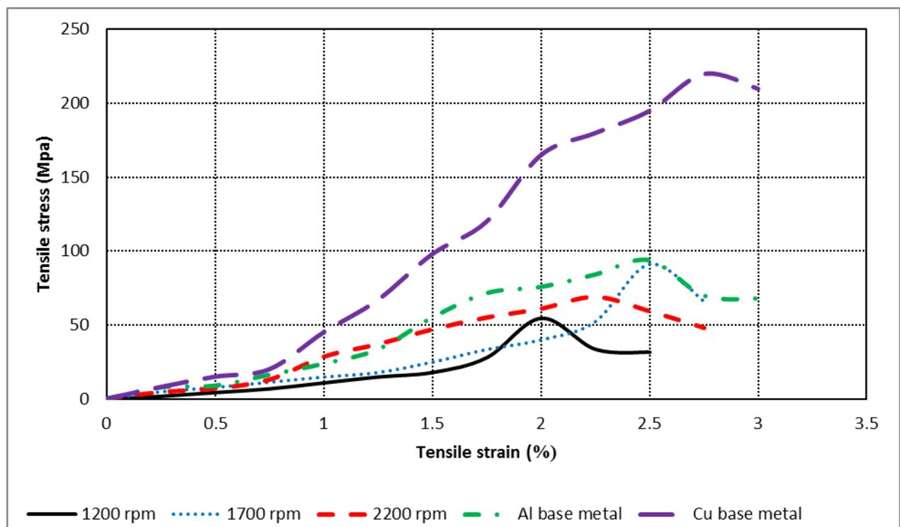
**Figure 9** Tensile test of the dissimilar Al-Cu welded joints at three different rotational speeds.
