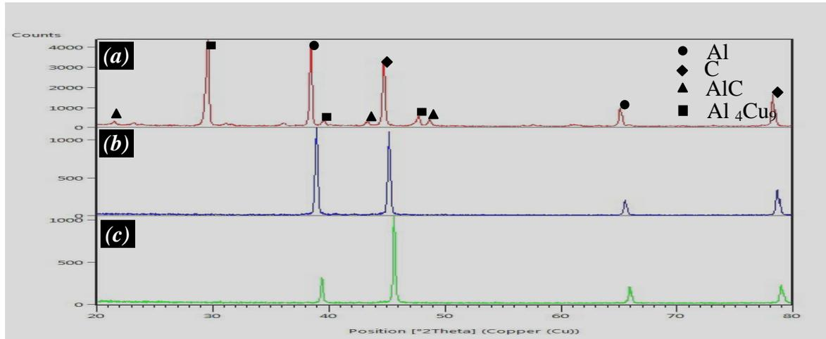
**Figure 6:** X-ray diffraction analysis of the welded joints FSW at: (a) rotational speed of 2200, (b) rotational speed of 1700 and (c) rotational speed of 1200 rpm.
