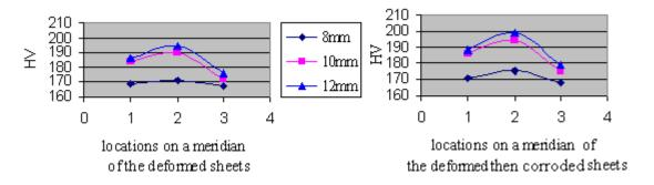
Figure (12). The hardness at points 1, 2 and 3 of a deformed non-corroded sheets (on the left) and the deformed then corroded sheets (on the right) for a biaxial strain path
