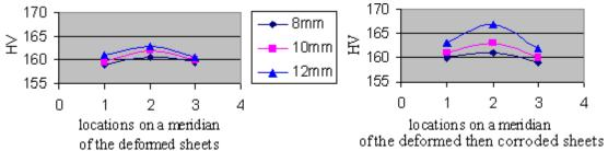
Figure (10). The hardness at points 1, 2 and 3 of a deformed non-corroded sheets (on the left) and the deformed then corroded sheets (on the right) for a uniaxial strain path
