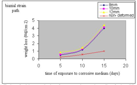
Figure (8). The loss of weight versus the time of exposure to the corrosive medium, for three different stain paths
