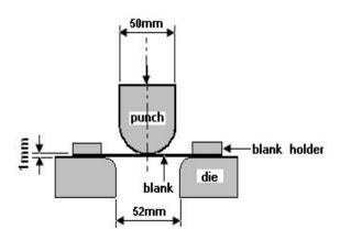
Figure (4): The stretching set up
