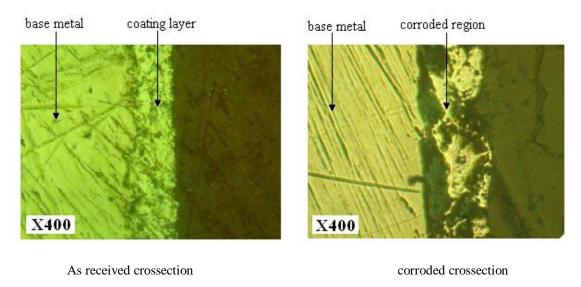
Figure (7). Micrograph showing the as received crossection and the corroded crossection of the HSLA steel sheet
