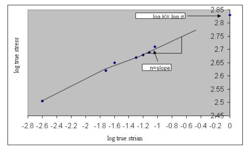
Figure (3). The log true stress- true strain diagram
