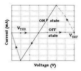
Fig.(1) I/V characteristics for SIS device, showing forward threshold voltage V<sub>THF</sub> and reverse threshold voltage V<sub>THR</sub> on the curve.
