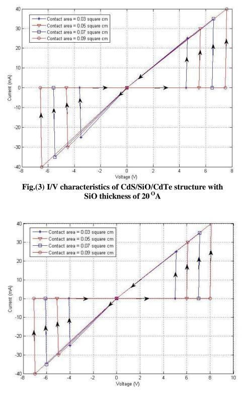
Fig.(4) I/V characteristics of CdS/SiO/CdTe structure with SiO thickness of 25  $^{\rm O}{\rm A}$
