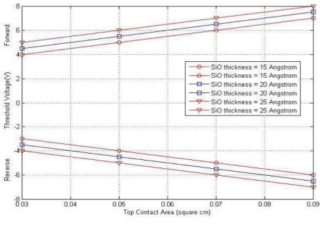
Fig.(6) threshold voltages versus top contact area of CdS/SiO/CdTe structure
