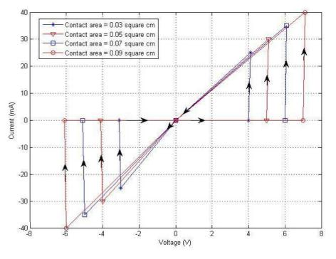
Fig.(2) I/V characteristics of CdS/SiO/CdTe structure with SiO thickness of 15  $^{\rm O}$ A
