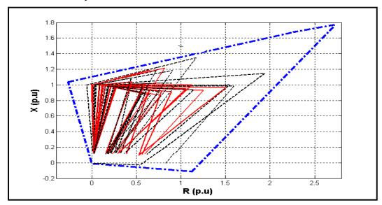
Figure (3) Resultant impedance characteristics for many transmission lines
