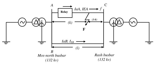
Figure (2): a section from northern Iraqi network (132kv)
