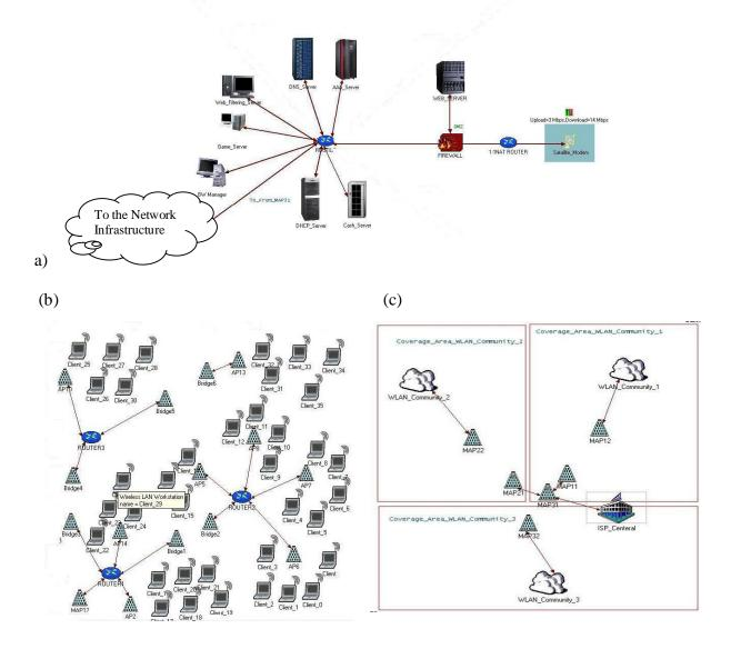
Fig. (1): Structure of WISP System: (a) ISP (Management) Center (b) Distribution Network (c) The Whole System
