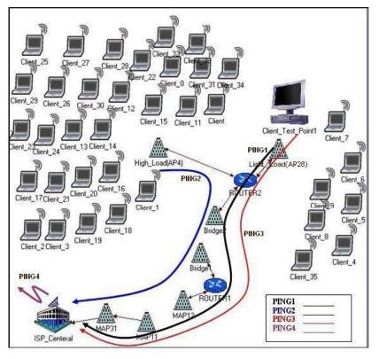
Fig. (7): Network Setup of Latency Measurements
