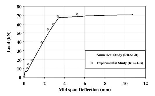
Figure (15): Numerical and Experimental Load/Deflection Curve of Beam Strengthened with One Layer of GFRP Sheets
