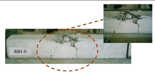
Figure (11): Failure mod of Beam (RB1-0)
