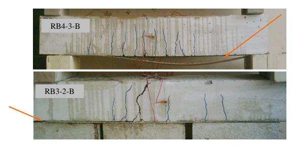
Figure (12): Failure mod of Beams (RB3-2-B) and (RB4-3-B)
