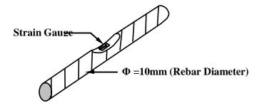
Figure (2): Homemade Internal Strain Gage
