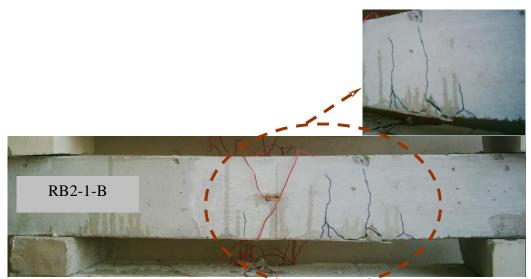
Figure (13): Failure mod of Beams (RB2-1-B)
