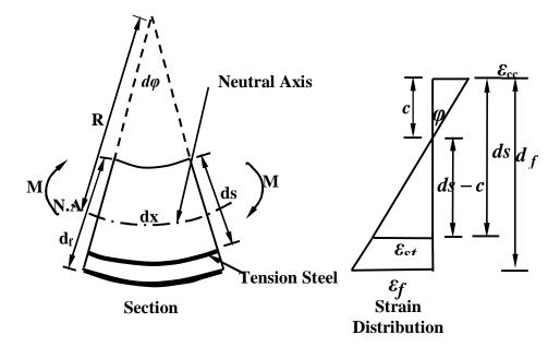
Figure (9): Rotation of Flexural Member
