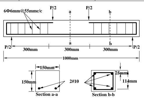
Figure (1): Test Beam Geometry
