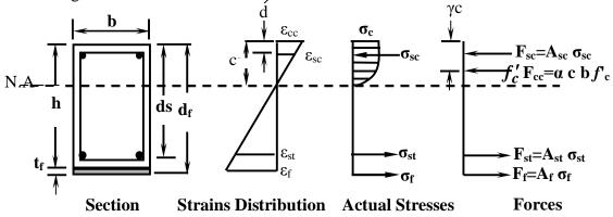
Figure (7): Strains, stresses, and forces used in the moment curvature model.
