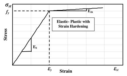
Figure (5): Theoretical Stress-Strain Plot of Steel Reinforcement
