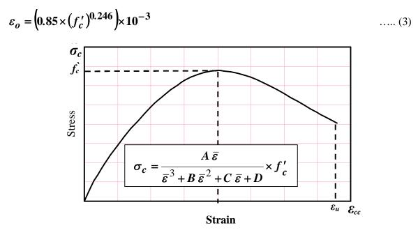
Figure (3): Schematic of concrete stress-strain behavior Developed Al-Sulayfani [10]
