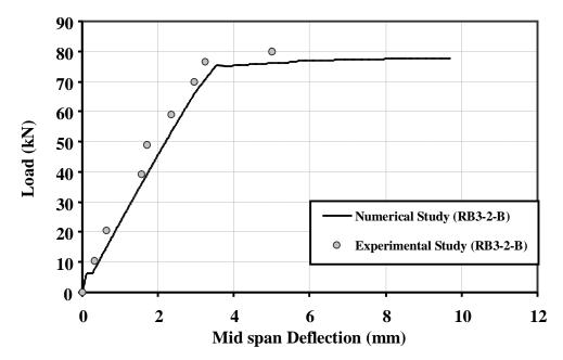
Figure (16): Numerical and Experimental Load/Deflection Curve of Beam Strengthened with Tow Layers of GFRP Sheets
