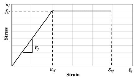
Figure (6): Average Stress-Strain Plot of GFRP
