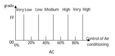
**Figure (8): Membership function of Air Conditioning Control (AC)**
