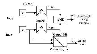
Figure (1): Sugeno Fuzzy Inference Engine Inp<sub>1</sub>, Inp<sub>2</sub>: Input<sub>1</sub> and Input<sub>2</sub> respectively Inp MF<sub>1</sub>, Inp MF<sub>2</sub>, Output MF: Memberships of Input<sub>1</sub>, Input<sub>2</sub>, and Output respectively
