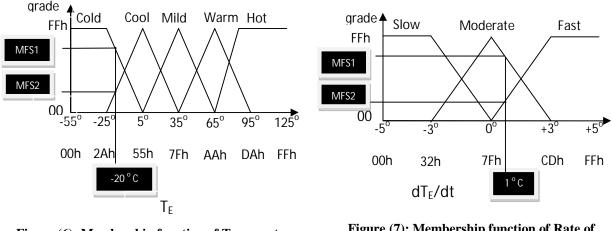
Figure (6): Membership function of Temperature Error  $(T_E)$
