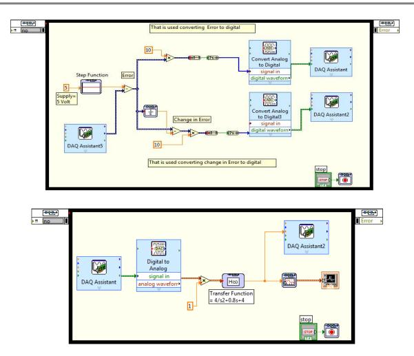
Figure (12): Block diagram of the Sugeno system using LabView
