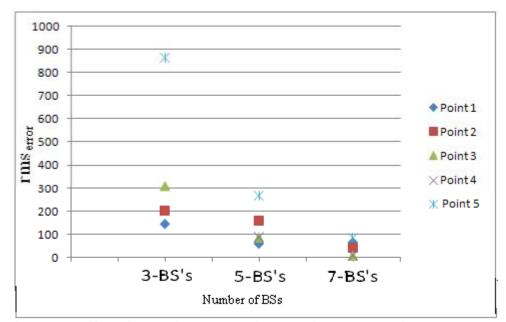
Fig. (5) The effect of increasing number of base stations on rms<sub>error</sub> in UMTS model.
