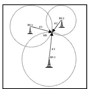
Fig. (2): Mobile positioning using three base stations
