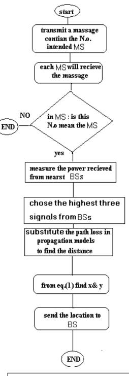
**Fig. (4)**: The flowchart of the location finding algorithm.
