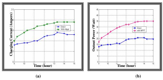
Figure (9): Measured a) charging current and b) output power with and without using Incremental conductance algorithm.
