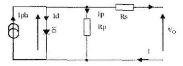
Figure (1): Simplified equivalent circuit of a solar cell.
