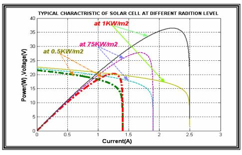
Figure (2): output I-V characteristics of a typical solar cell under different Radiations.
