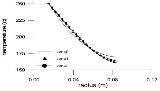
Figure (2) Temperature distribution along the fin
