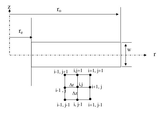
Figure (1) the dimensions of annular fin constant thickness
