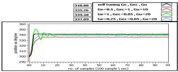
Figure 11: Control tracking response for a step from 300° to 340°
