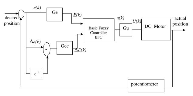
Figure 1: Block diagram of fixed factors fuzzy controller
