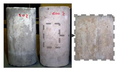
Fig (5) Color surface and micro cracks at 600 °C.
