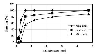
Fig (1): Sieve analysis of fine aggregate
