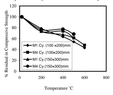
Fig. (9) Residual compressive strength of M1 and M4 with two specimens size of cylinder
