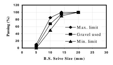
Fig (2): Sieve analysis of coarse aggregate
