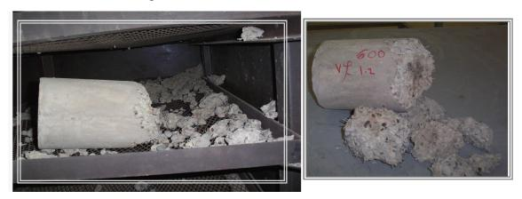
Fig. (12) Explosive spalling
