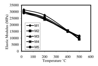
Fig (13): Residual modulus of elasticity
