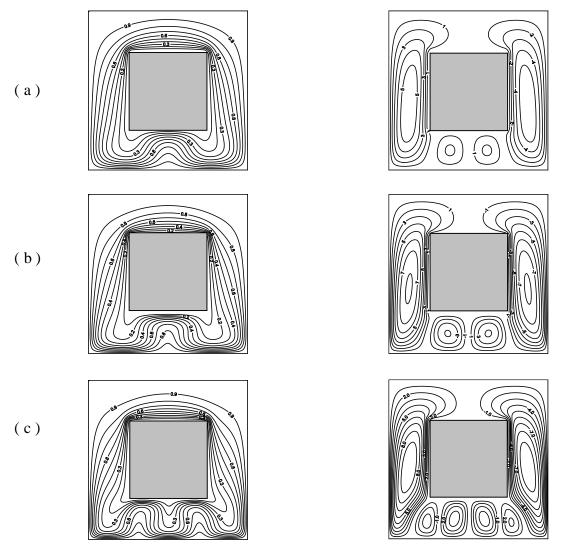
Fig ( 3 ) Isotherms lines & Stream functions for  $e_x = 0$ ,  $e_y = 0$ ,  $L_b = 0.5$  (a) Ra=200 , (b) Ra=300, (c) Ra=400
