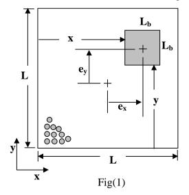
The body is maintained at constant uniform cold temperature and walls of cavity maintained at constant cold temperature. The governing equations that describe the heat transfer process for steady natural convection with Darcy flow and Boussinesq approximation with ( continuity , momentum and energy ) equations are as follows:
