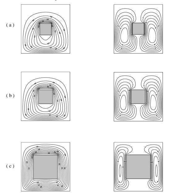
Fig ( 4 ) Isotherms lines & Stream functions for  $e_x = 0$ ,  $e_y = 0$ , Ra = 100 (a)  $L_b=0.25$ , (b)  $L_b=0.3$ , (c)  $e_y=L_b=0.5$
