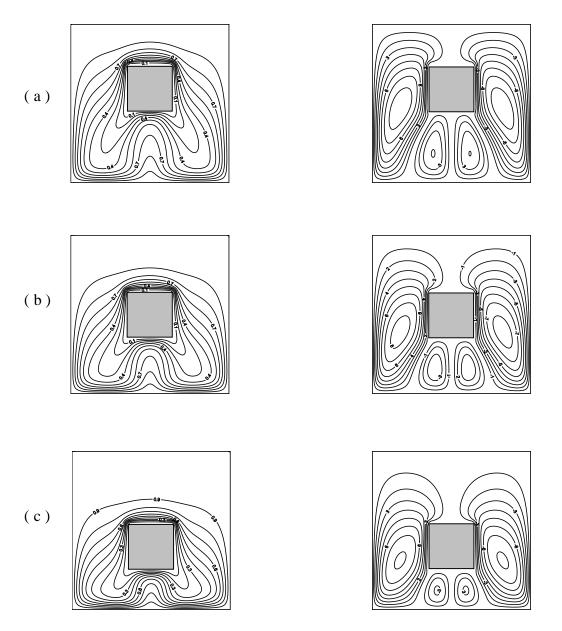
Fig ( 5 ) Isotherms lines & Stream functions for  $~L_b=0.3$  ,  $e_x=0$  , Ra=300 (a)  $e_y{=}0.1$  , (b)  $e_y{=}0,$  (c)  $e_y{=}$  -0.1
