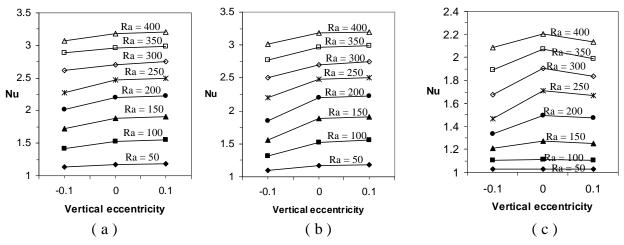
Fig (8) Nu versus  $e_v$  for  $e_x=0$  (a)  $L_b=0.25$ , (b)  $L_b=0.3$ , (c)  $L_b=0.5$
