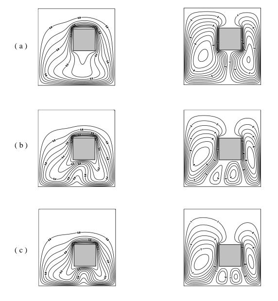
Fig ( 6 ) Isotherms lines & Stream functions for  $L_b=0.3$ ,  $e_x=0.1$ , Ra=300 (a)  $e_y=0.1$ , (b)  $e_y=0$ , (c)  $e_y=-0.1$
