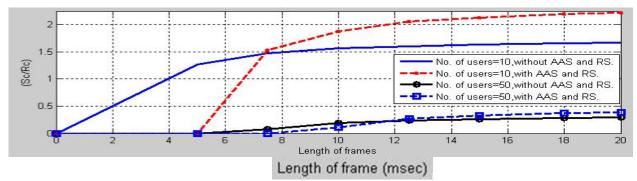
Figure (15) Shows Sc/Rc versus length of frames for two values of number of users.
