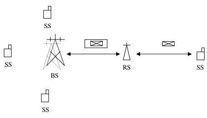
Figure (2) WiMAX network with Relay Station .
