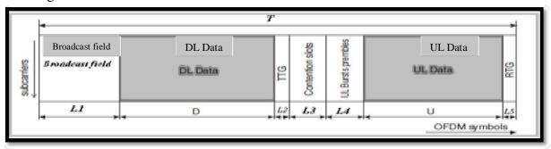
Figure (6) Details of OFDM symbols used for data(without RS and AAS).
