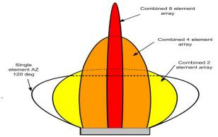
Figure (4) Single, 2, 4 and 8 Element Performance Illustration[6]
