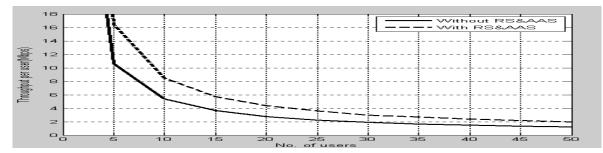
Figure (16) Throughput per user with and without AAS and RS.
