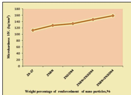
Figure 5: Micro hardness values of ZA-27 alloy and its composites
