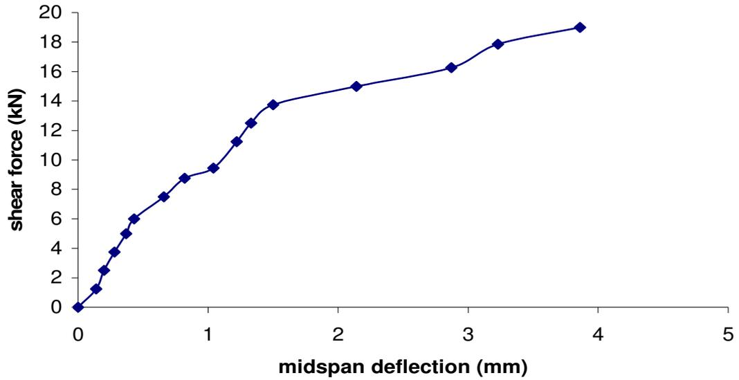
**Fig.(4) Midspan deflection for Monopanel Specimen with H=400mm**
