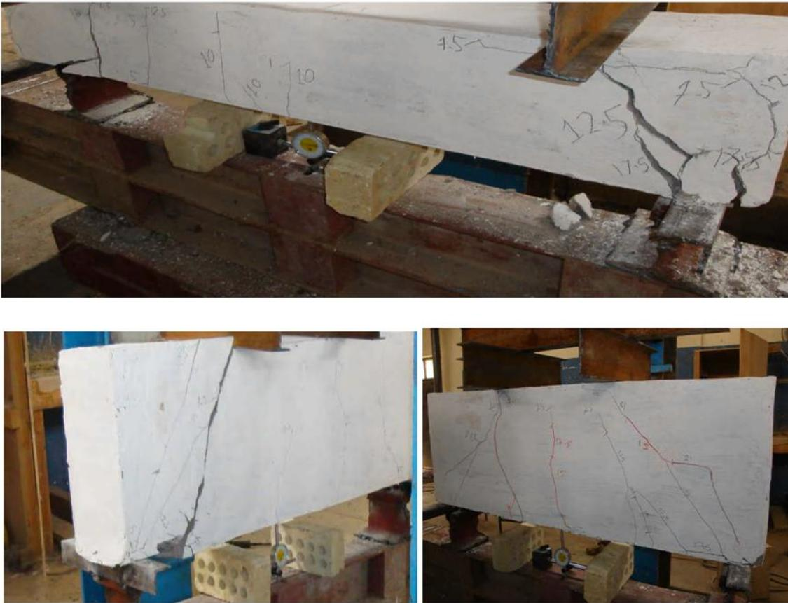
**Fig.(6)Shear crack pattern for Monopanel beam specimens**
