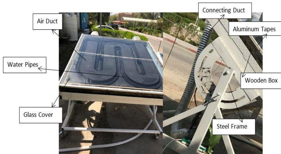
Fig. (1) The Test Rig
