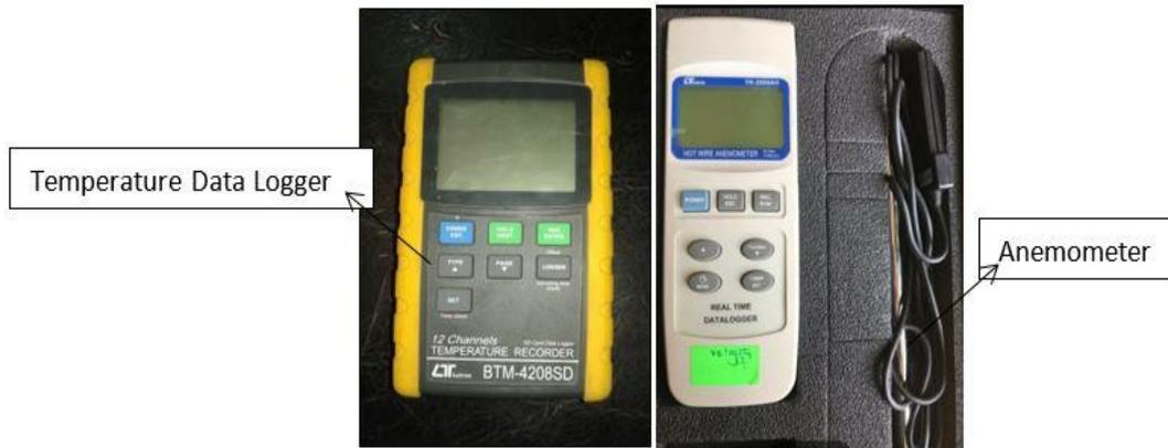
Fig. (2) The Measurement Devices
