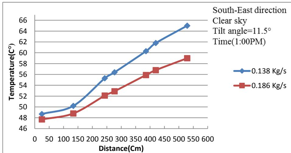
**Fig (8) Mass Flow Rate Effect on the Air Temperature**
