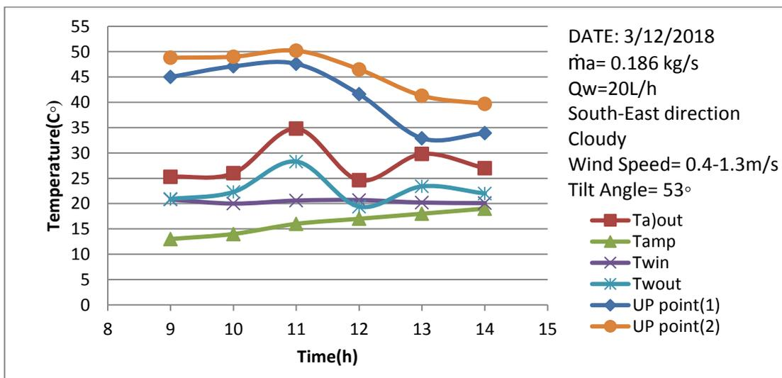
**Fig. (4) Variation of Temperatures with Time for Cloudy Condition**
