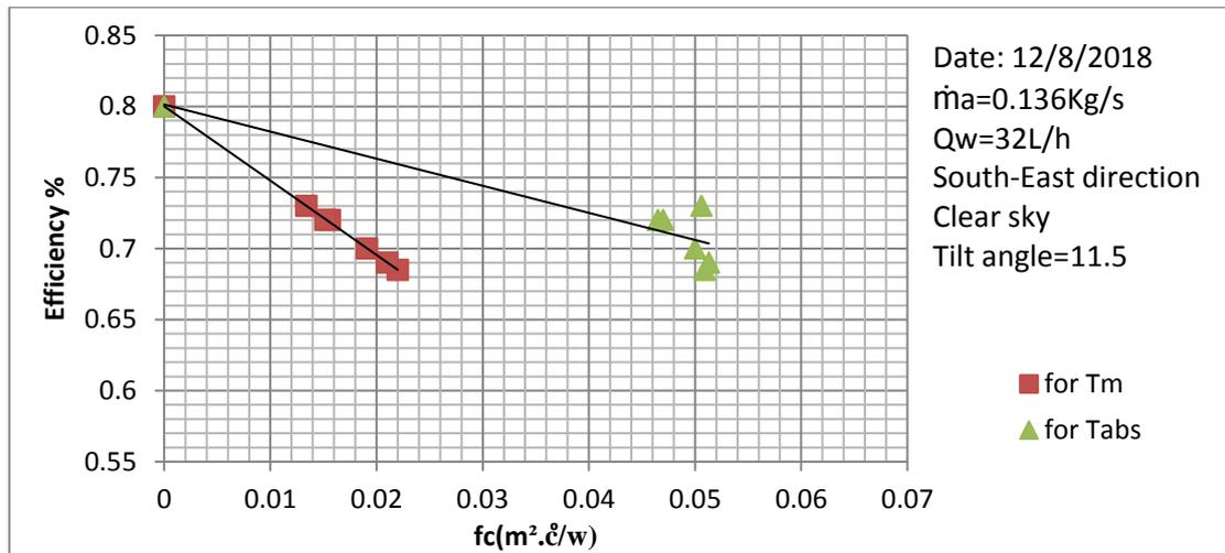
**Fig (10) Performance Curve of the Collector**
