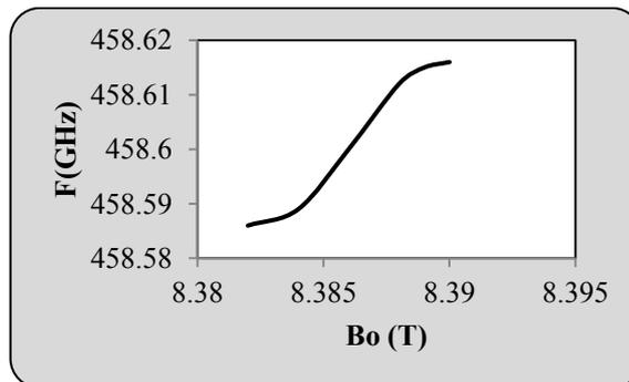
Figure 6: Frequency of the TE<sub>0,6</sub>–mode as a function of mode with the main magnetic field
