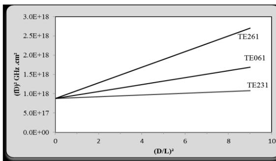
Figure 4: indicates the competing second harmonic (TE<sub>061</sub> and TE<sub>261</sub>) modes with the dominant mode in gyrotron at 460 GHz.
