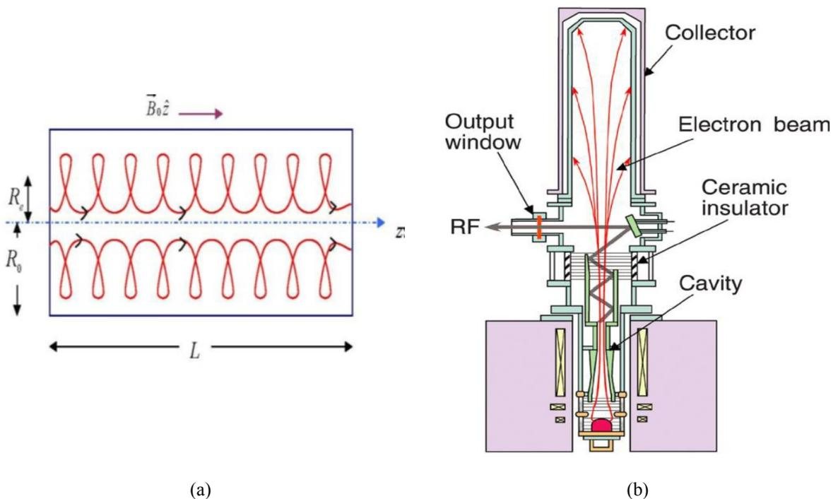
**Figure 1: (a) Single cavity of the gyrotron [10], (b) The gyrotron cavity**
