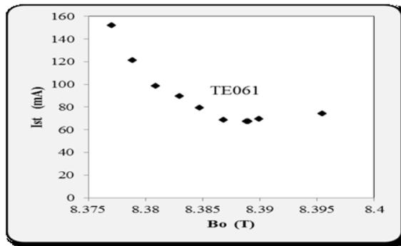
Figure 2: Start oscillation current data versus flux density for second harmonic TE<sub>061</sub> mode from in the range (8.3T to 8.4T)
