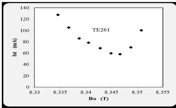
Figure 3: Start oscillation current data versus magnetic flux density for second harmonic TE<sub>261</sub> mode from (8.33T to 8.355T)
